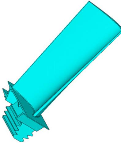
Figure 3: The geometric model of the turbine blade
