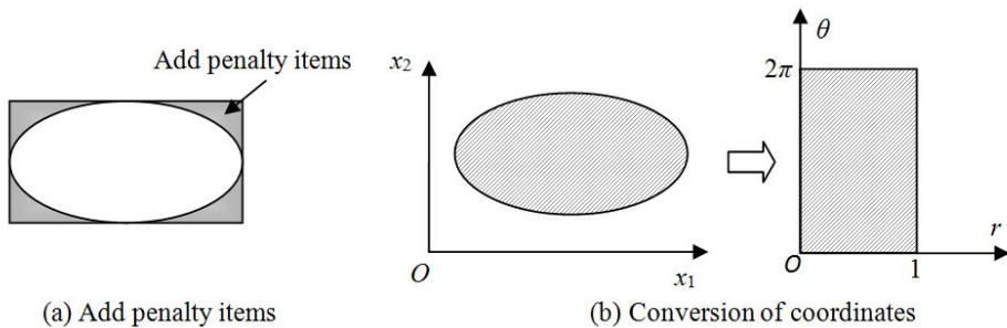
Figure 2: Two methods for imposing the hyper-ellipsoidal constraint
