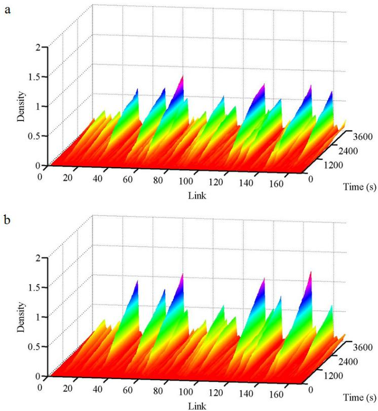
Figure 6: Link density. (a) is for case I: 25% vehicles disobey the navigation commands. (b) is for case II: 50% vehicles disobey the navigation commands.
