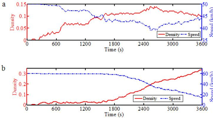
Figure 4: Samples of the consistency between density and speed on a link. (a) is for link 50. (b) is for link 135 in the case of Fig. 3 (b).
