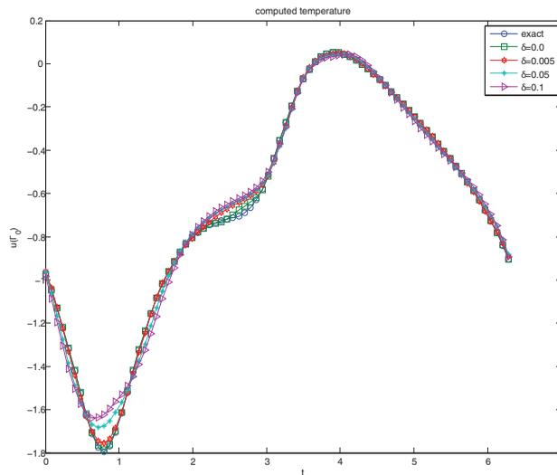
Figure 4: Ex.2. Regularization parameters  $\lambda = 2.5e - 15, 0.0012, 0.0044, 0.0062$  for the cases of  $\delta = 0, 0.005, 0.05, 0.1$ , respectively.
