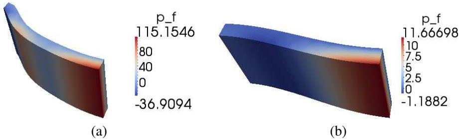
Figure 15: The deformed meshes for dynamic simulation with pore water for hold (a) and impulse (b) loadings (with inertia terms).  $p_f$  units in Pa.
