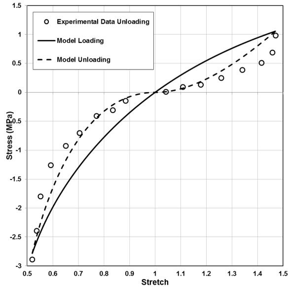
Figure 5: Experimental data [6] plotted against the proposed model for the unloading response of rubber using damage function at a strain-rate of 0.01 mm/mm/s.
