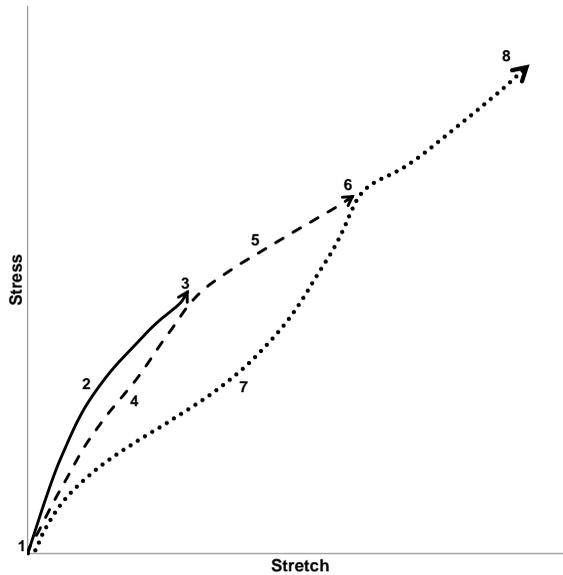
Figure 1: Mullins' effect schematic representation.
