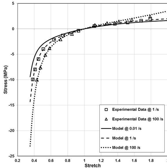
Figure 4: Experimental data [6] plotted against the proposed model for the dynamic response of rubber at a strain-rate of 0.01, 1.0 and 100.0 mm/mm/s.
