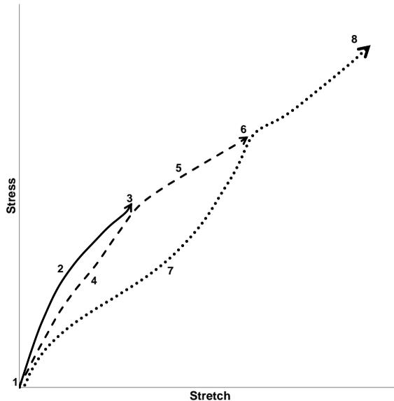
Figure 1: Mullins' effect schematic representation.
