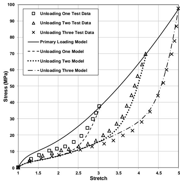
Figure 8: Experimental unloading data [17] plotted against the proposed model for Mullins' effect with third maximum stretch.
