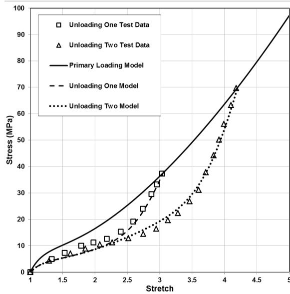
Figure 7: Experimental unloading data [17] plotted against the proposed model for Mullins' effect up to second maximum stretch.
