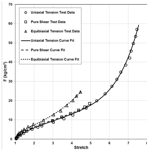
Figure 2: Experimental data [19] for 8% S rubber in uniaxial tension, pure shear and equibiaxial tension fitted to the three-term Ogden model.
