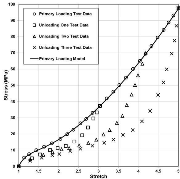
Figure 6: Experimental loading data [17] plotted against the hyperelastic three-term Ogden model for primary response of rubber compound.
