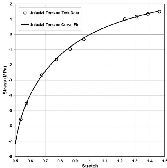
Figure 3: Experimental data [6] plotted against the proposed model for the quasi-static response of rubber at a strain-rate of 0.01 mm/mm/s.
