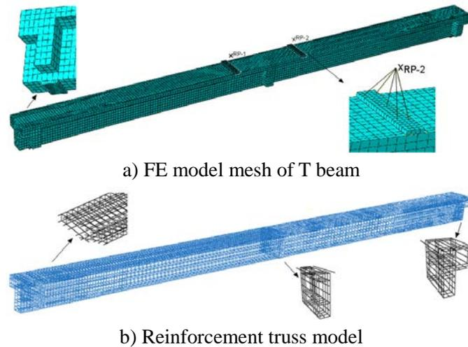
**Figure 4:** Finite element model of T-beam
