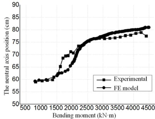
**Figure 12:** Neutral axis position-midspan moment curve
