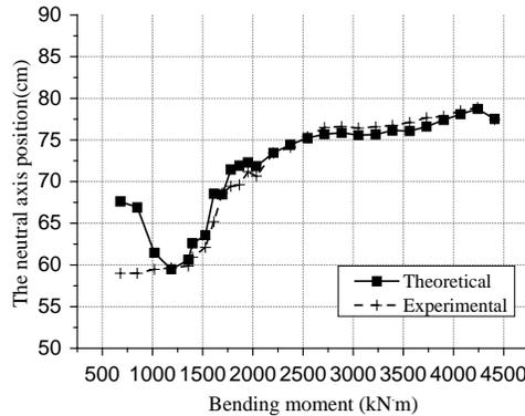
**Figure 15:** Neutral axis position-mid span moment curve
