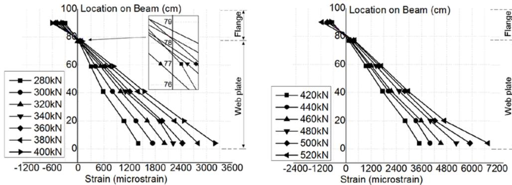
**Figure 11:** Mid-span section strain analysis
