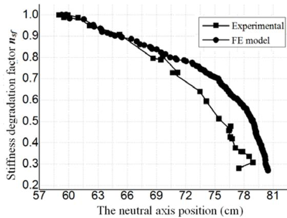
**Figure 13:** Stiffness degradation factor-neutral axis position curve
