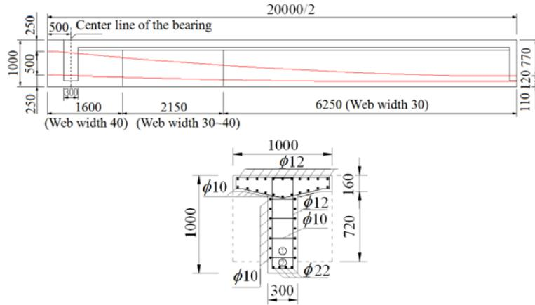
**Figure 1:** Structure and reinforcement diagram of prestressed concrete T-beam/mm
