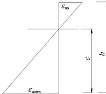
**Figure 14:** Strain diagram of plane section
