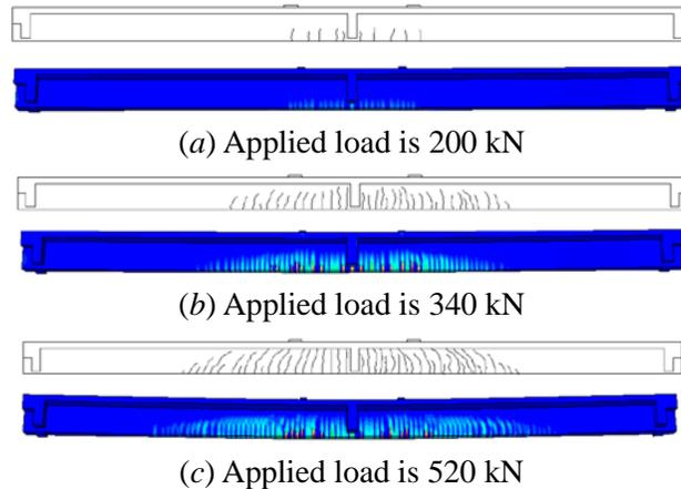
**Figure 16:** Tensile plastic strain cloud images of finite element model
