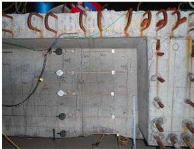
**Figure 10:** Micrometer gauge layout
