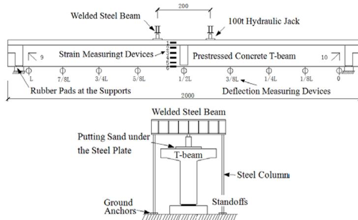
**Figure 3:** T-beam test loading device and measuring points setup/cm
