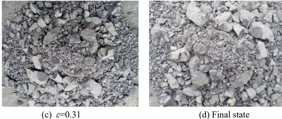
**Figure 9:** State of fragmentation in each stage after compression of #1
