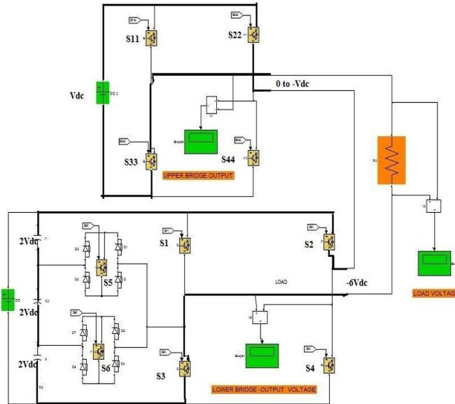
Figure n: Mode 14 operation of the proposed inverter
