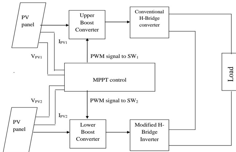
**Figure 1:** Block diagram of the proposed inverter
