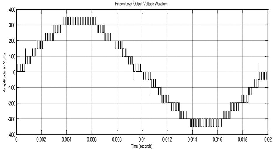
**Figure 12:** Fifteen level inverter output voltage
