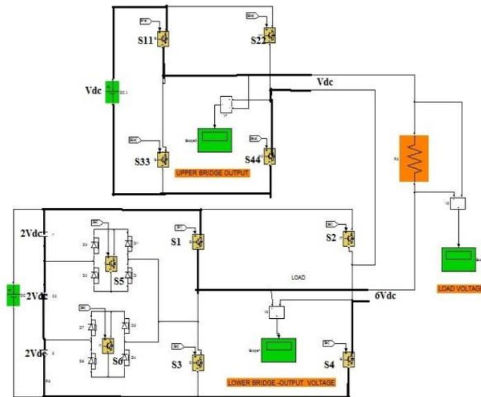
**Figure a:** Mode 1 operation of the proposed inverter
