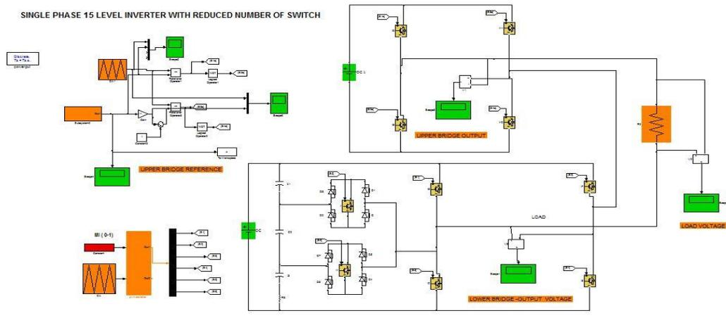
**Figure 7:** Simulink model of fifteen level inverter
