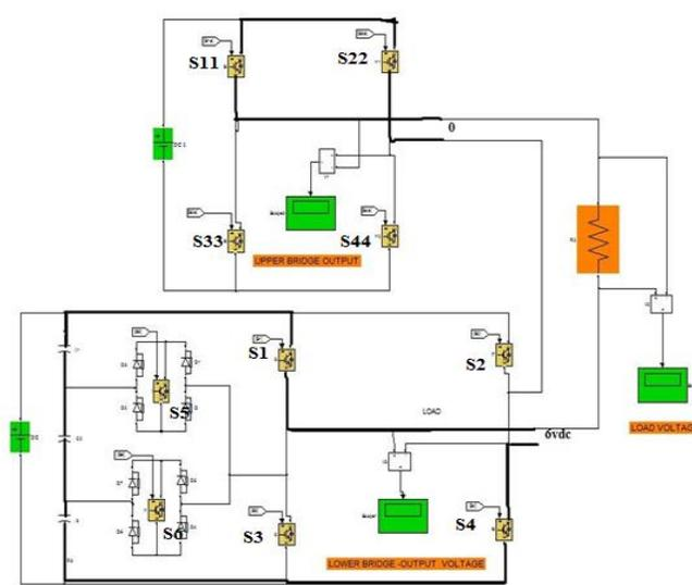
**Figure b:** Mode 2 operation of the proposed inverter
