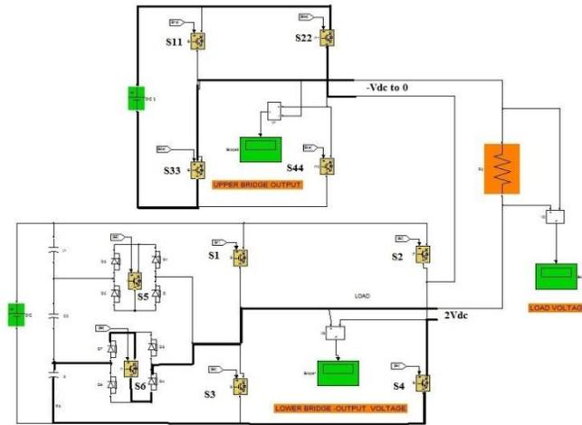
**Figure f:** Mode 6 operation of the proposed inverter
