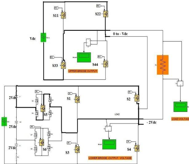
**Figure j:** Mode 10 operation of the proposed inverter
