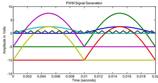
**Figure 4:** PWM signal generation of lower inverter
