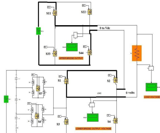
**Figure g:** Mode 7 operation of the proposed inverter
