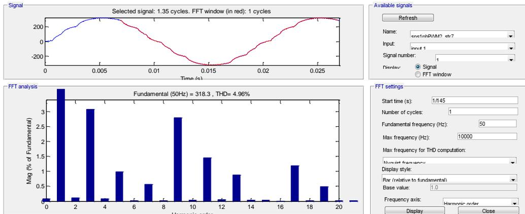
**Figure 18:** THD analysis of grid connected fifteen level inverter
