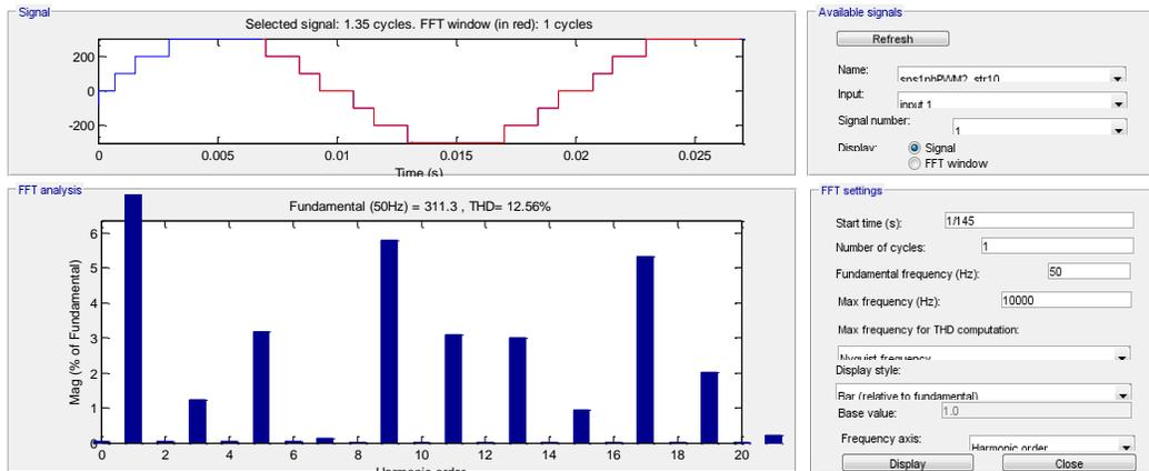
**Figure 17:** THD analysis of seven level inverter
