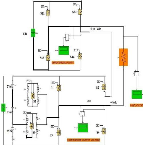
**Figure l:** Mode 12 operation of the proposed inverter
