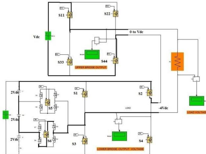
**Figure k:** Mode 11 operation of the proposed inverter
