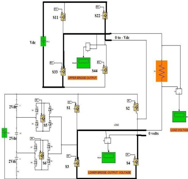
**Figure h:** Mode 8 operation of the proposed inverter
