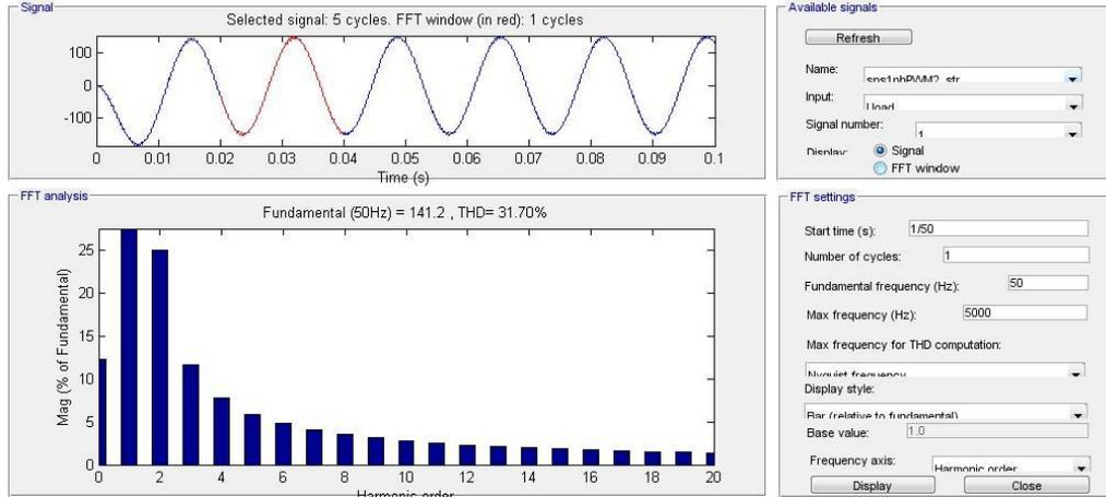
**Figure 16:** THD analysis of three level inverter
