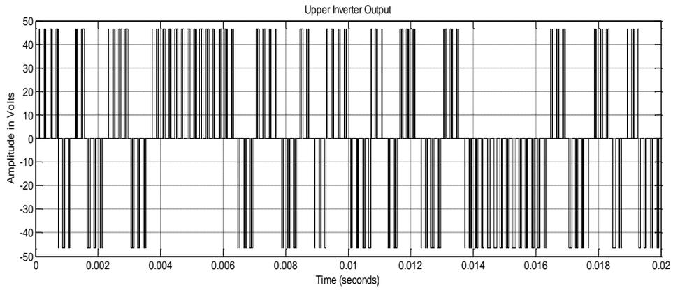
**Figure 10:** Upper inverter output voltage
