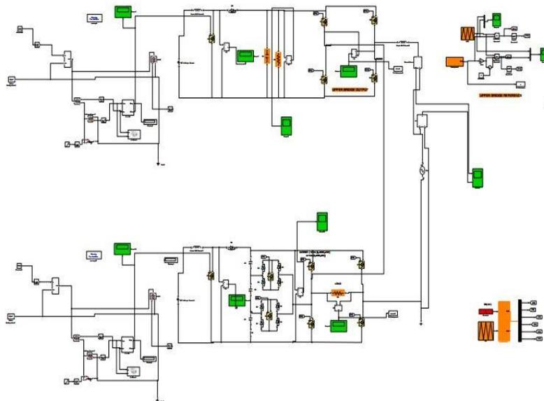
**Figure 13:** Simulink model of grid connected fifteen level inverter for PV system
