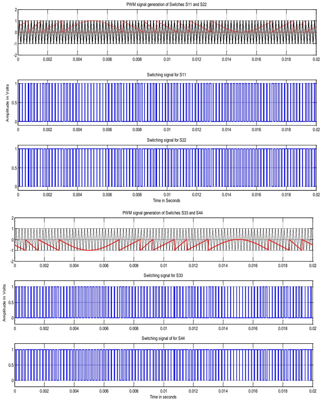
**Figure 9:** Switching signal of upper inverter
