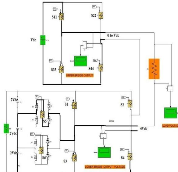
**Figure c:** Mode 3 operation of the proposed inverter
