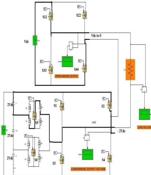
**Figure i:** Mode 9 operation of the proposed inverter
