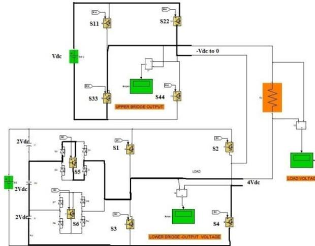
**Figure d:** Mode 4 operation of the proposed inverter
