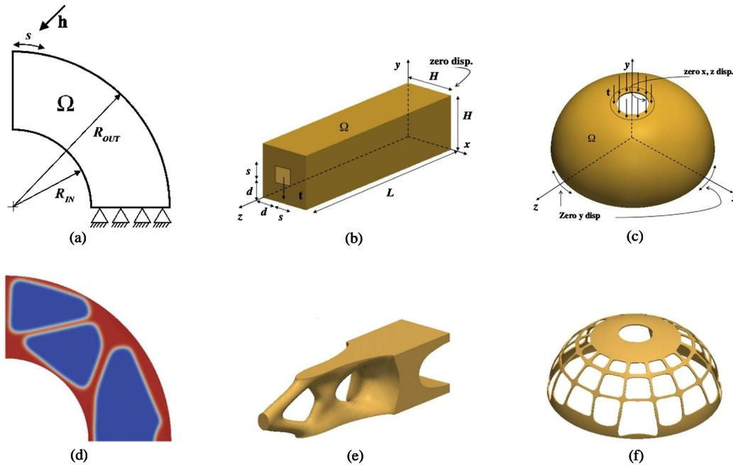
**Figure 14:** Numerical examples of the ITO using the phase field model: (a) Design domain of the 2D example, (b) Design domain of the 3D example, (c) Design domain of the thin shell example, (d) Optimization result of the 2D example, (e) Optimization result of the 3D example, and (f) Optimization result of the thin shell example [Dedè, Borden and Hughes (2012)]
