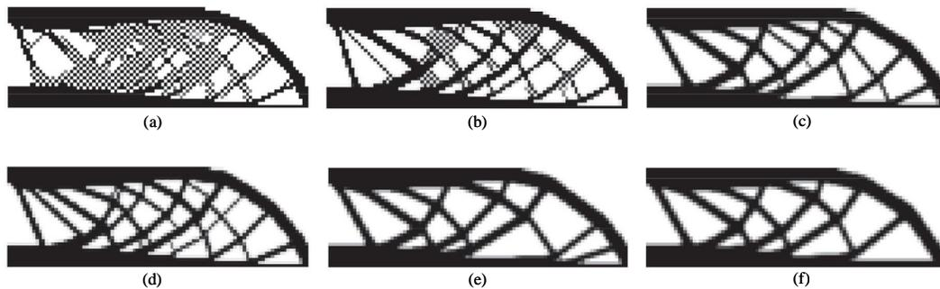
**Figure 8:** Mesh dependence caused by the B-spline orders: (a)  $p = q = 2$ , (b)  $p = q = 4$ , (c)  $p = q = 5$ , (d)  $p = q = 6$ , (e)  $p = q = 7$ , (f)  $p = q = 9$  [Qian (2013)]
