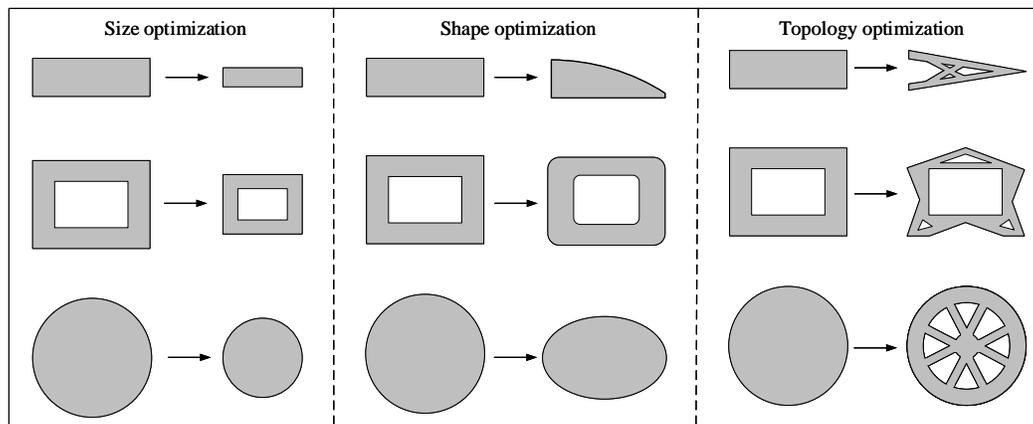
**Figure 1:** An illustration of structural optimization
