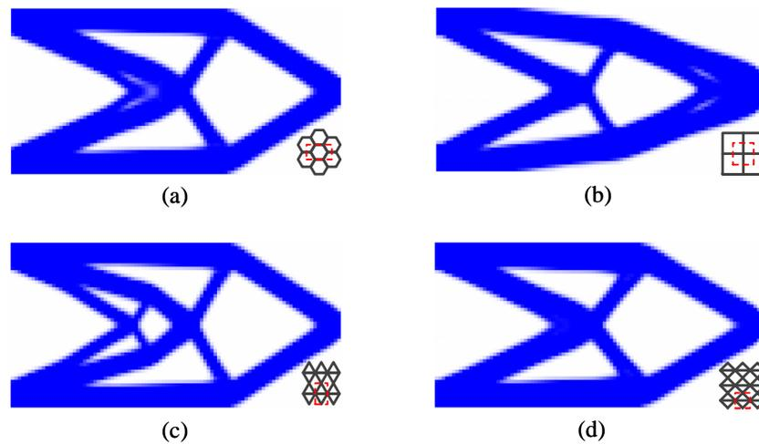
**Figure 11:** The optimization results of the cantilever beam: (a) Hexagon lattice, (b) Square lattice, (c) Acute triangle lattice and (d) Obtuse triangle lattice [Wang, Xu and Pasini (2017)]
