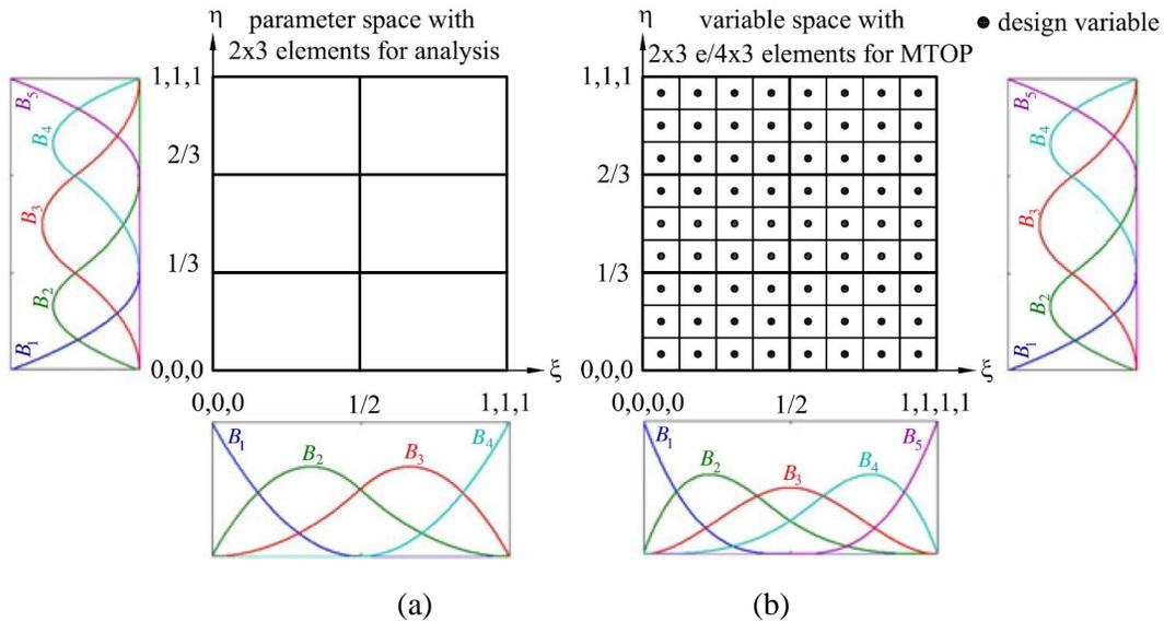
**Figure 9:** The parameter space and variable space of MTOPT: (a) Discretization in parameter space and the basis functions for analysis, and (b) Discretization in variable space and the basis functions for MTOPT [Lieu and Lee (2017b)]
