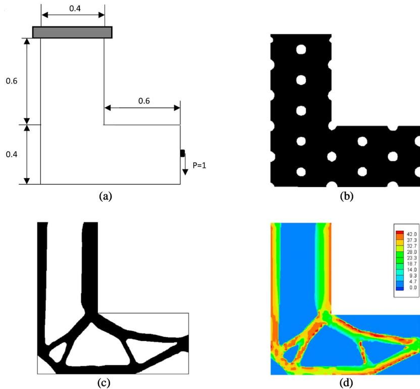
**Figure 13:** The level-set-based ITO of the L-shape structure: (a) Design domain and boundary conditions, (b) Initial topology, (c) Optimization result and (d) Von Mises stress contour [Ghasemi, Park and Rabczuk (2017)]
