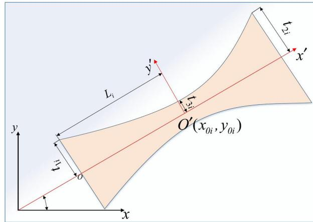
**Figure 15:** Geometry description of the  $i$ th component with straight skeleton and quadratically variable thicknesses [Xie, Wang, Xu et al. (2018)]
