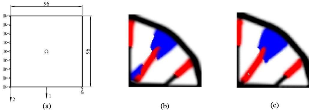
**Figure 10:** Optimized topologies of the bride structure: (a) Design domain and boundary condition, (b)  $96 \times 96$  elements without subelements,  $c = 49.5033$ , and (c)  $32 \times 32$  elements with  $3 \times 3$  subelements in each element,  $c = 47.8111$  [Lieu and Lee (2017b)]
