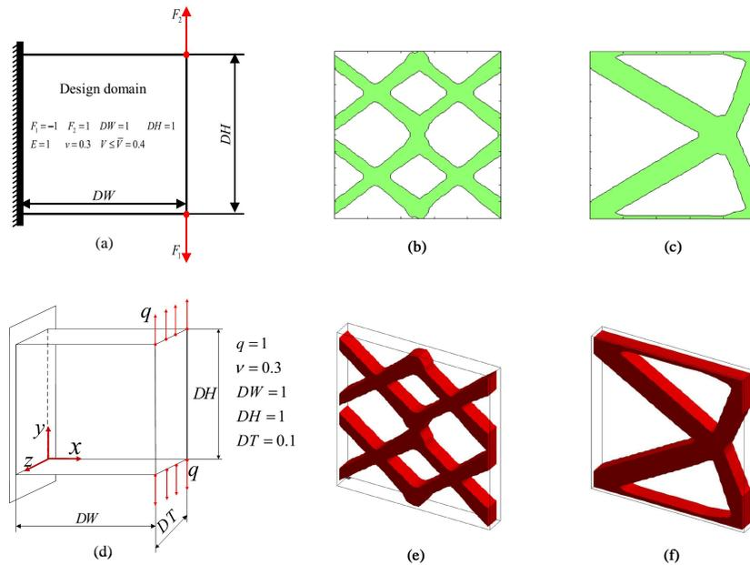
**Figure 16:** Numerical examples of the MMC-based ITO: (a) Design domain of the 2D example, (b) Initial design of the 2D example, (c) Optimization result of the 2D example, (d) Design domain of the 3D example, (e) Initial design of the 3D example and (f) Optimization result of the 3D example [Xie, Wang, Xu et al. (2018)]
