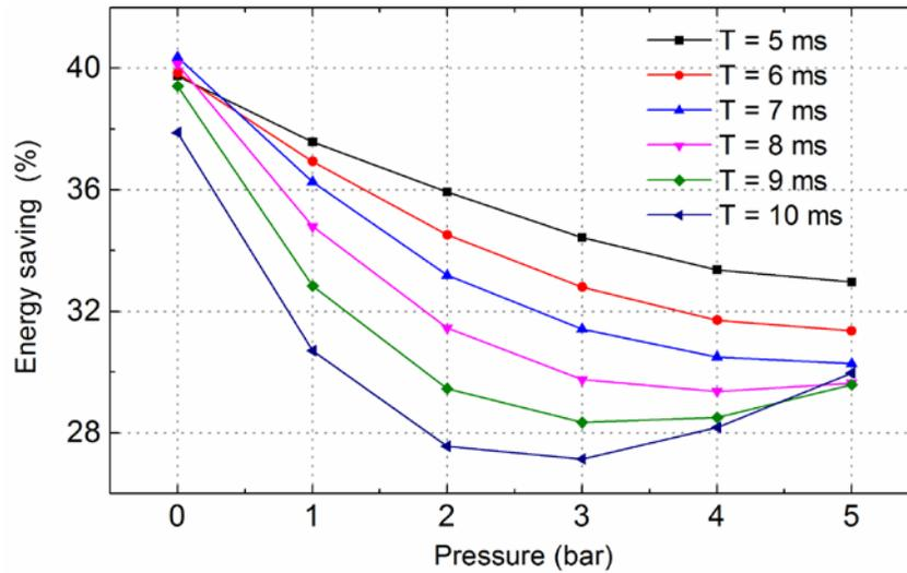
**Figure 13:** energy-saaving efficiencies of the EMVT system
