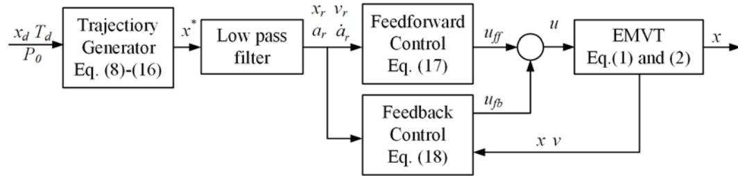
**Figure 4:** The structure diagram of the tracking controller
