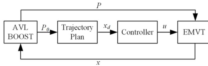
**Figure 14:** The structure of the co-simulation framework
