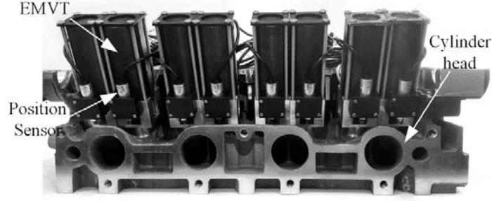
**Figure 1:** Prototype of EMVT
