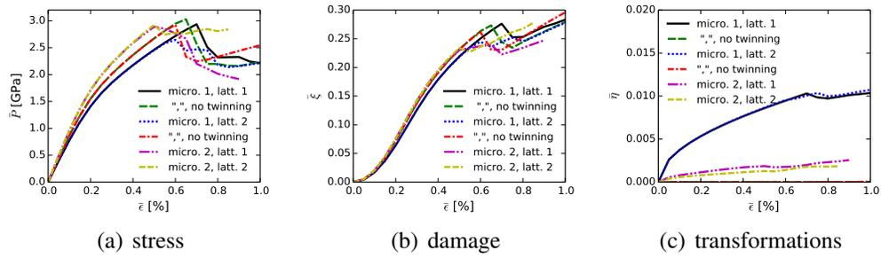
**Figure 6:** Averaged results for diamond-SiC versus applied shear strain  $\bar{\epsilon}$ : (a) shear stress  $\bar{P}$  (b) fracture  $\bar{\xi}$  (c) twinning  $\bar{\eta}$
