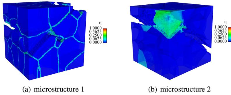
**Figure 5:** C-SiC, lattice 1, shear strain  $\bar{\epsilon} = 0.9\%$ : (a)  $V_2 = 0.20$ , (b)  $V_2 = 0.10$
