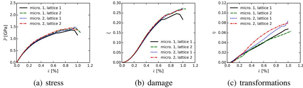
**Figure 3:** Averaged results for  $B_4C$ - $TiB_2$  versus applied shear strain  $\bar{\epsilon}$ : (a) shear stress  $\bar{P}$  (b) fracture  $\bar{\xi}$  (c) twinning, phase change, or slip  $\bar{\eta}$
