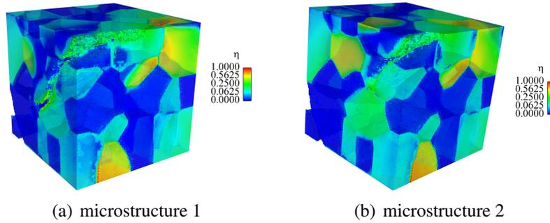
**Figure 2:**  $B_4C$ - $TiB_2$ , lattice 1, shear strain  $\bar{\epsilon} = 1\%$ : (a)  $V_2 = 0.10$  (b)  $V_2 = 0.18$
