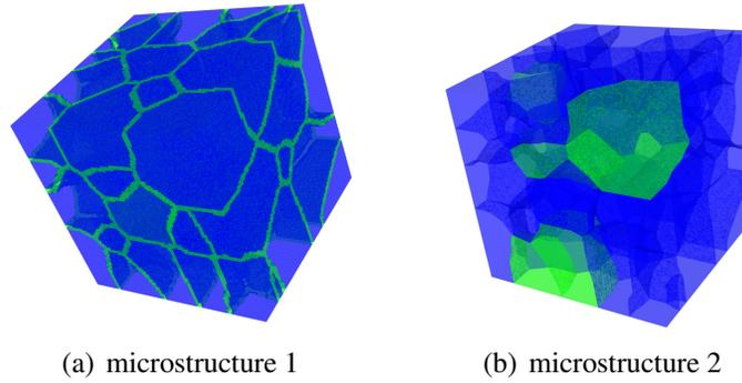
**Figure 4:** FE meshes; (C, SiC) crystals are (blue, green) and  $V_2$  is the volume fraction of SiC: (a) microstructure 1,  $V_2 = 0.20$  (b) microstructure 2,  $V_2 = 0.10$
