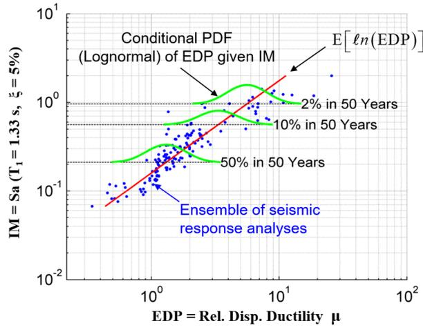
**Figure 6:** Conditional seismic demand hazard analysis result for EDP=relative displacement ductility
