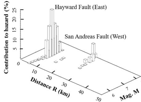
**Figure 5:** M-R deaggregation of the probabilistic seismic hazard corresponding to a probability of exceedance of 2% in 50 years ( $PE_{50}=2\%$ )
