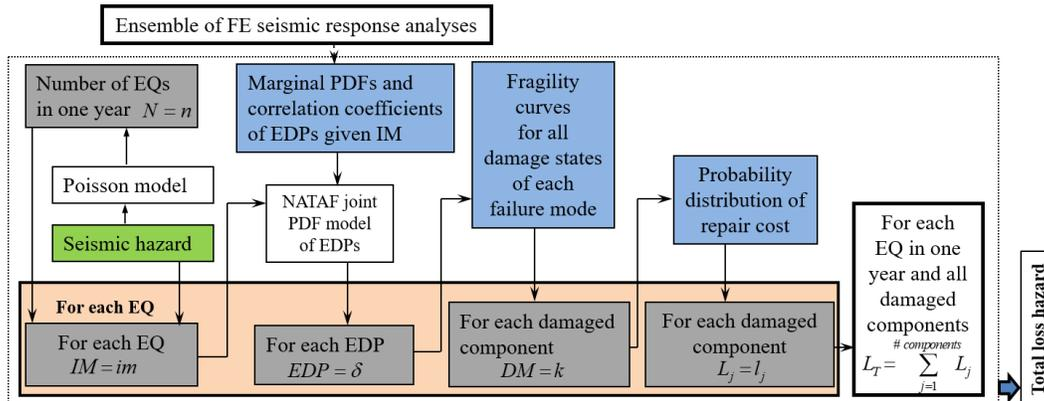
**Figure 10:** Flowchart of Multilayer Monte Carlo Simulation (MMCS) method for total loss hazard calculation
