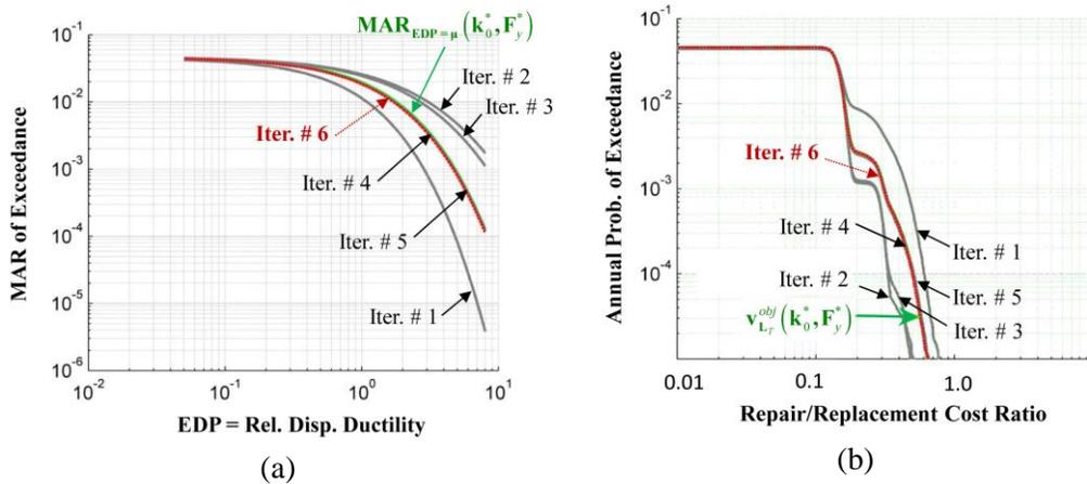
**Figure 16:** Evolution of the PBEE evaluation results during the optimization process: (a) probabilistic seismic demand hazard curves, and (b) probabilistic seismic loss hazard curves
