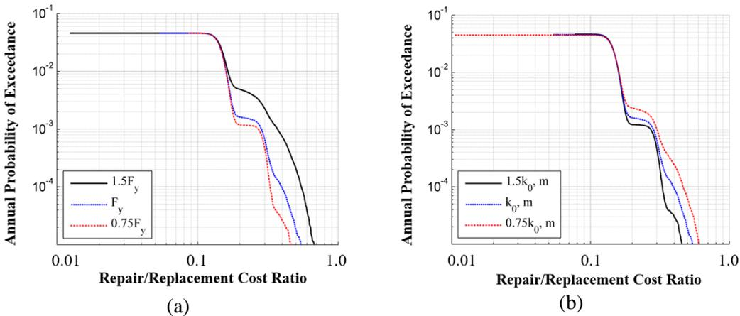
**Figure 13:** Probabilistic seismic loss hazard curves for SDOF systems with (a) different yield strengths, and (b) different initial stiffnesses
