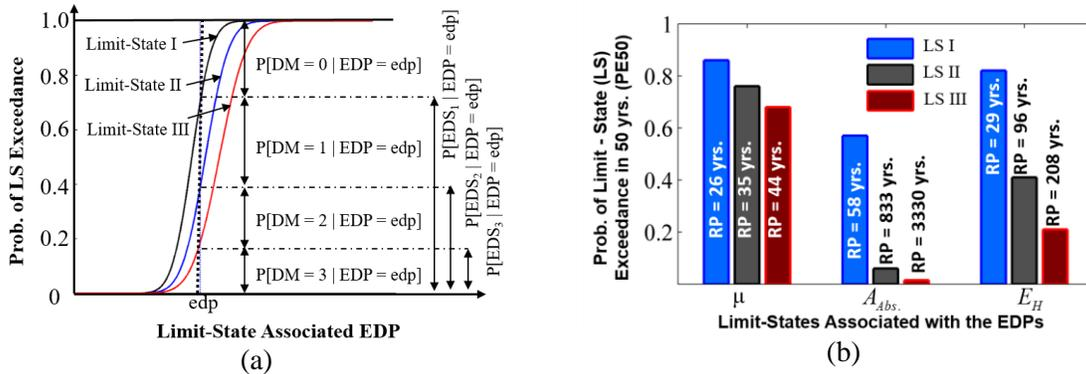
**Figure 8:** (a) Illustration of the probabilistic capacity curves and definition of conditional probability of damage states given EDP, and (b) seismic damage hazard results for the damage (or limit-) states associated with the EDPs considered for the illustrative example
