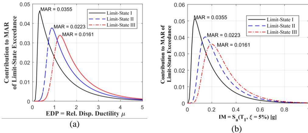
**Figure 9:** Damage hazard deaggregation with respect to (a) EDP and (b) IM for different damage/limit-state exceedances associated with EDP=relative displacement ductility (values of MAR of exceedance are indicated for each limit-state)
