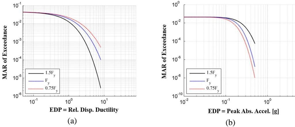
**Figure 12:** Probabilistic seismic demand hazard curves for: (a) relative displacement ductility, and (b) peak absolute acceleration of SDOF systems with different yield strengths
