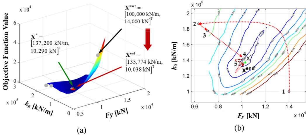
**Figure 15:** Optimization path for the PPBOSD illustrative example: (a) 3D plot, and (b) contour plot of the objective function
