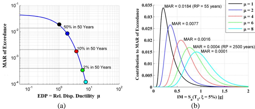
**Figure 7:** (a) Probabilistic seismic demand hazard curve for the relative displacement ductility (solid circles denoted for the points to be deaggregated), and (b) deaggregation of demand hazard points shown in Fig. 7(a) with respect to the intensity measure IM
