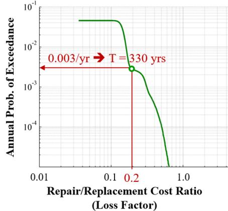
**Figure 11:** Probabilistic seismic loss hazard curve
