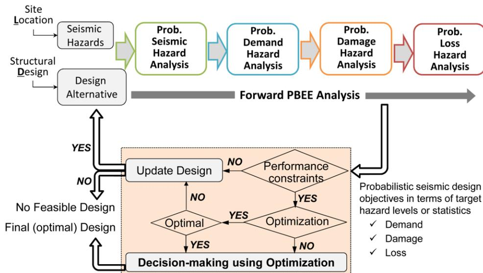
**Figure 3:** Probabilistic performance-based optimum seismic design (PPBOSD) framework
