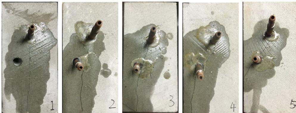
**Figure 5:** Resulting hydro-fractures with different pressures in No. 2 holes. The crack gradually turns to the direction of the No. 2 hole as the water pressure in the No. 2 hole increases
