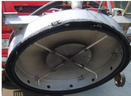
**Figure 1:** Structure of surface cleaner [Peng and Zhang (2018)]
