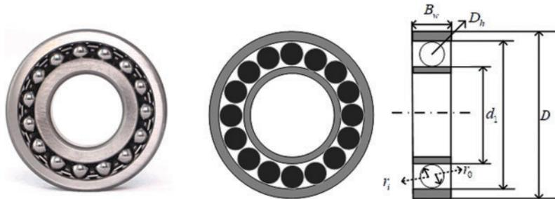
Figure 11: Schematic diagram of rolling element bearing design problem
