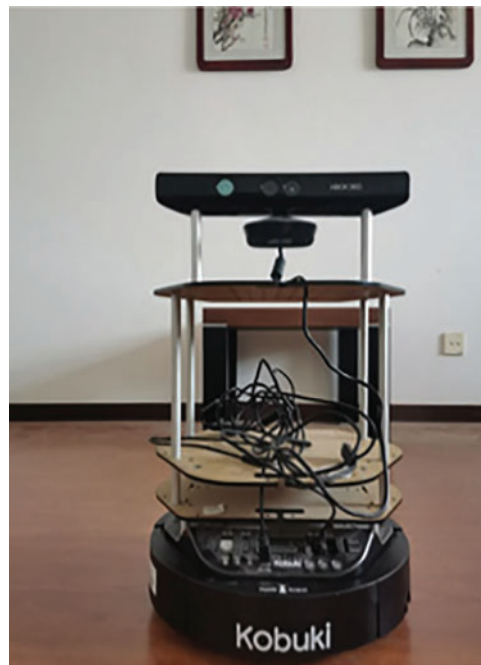
Figure 8: Mobile robot equipped with Kinect camera
