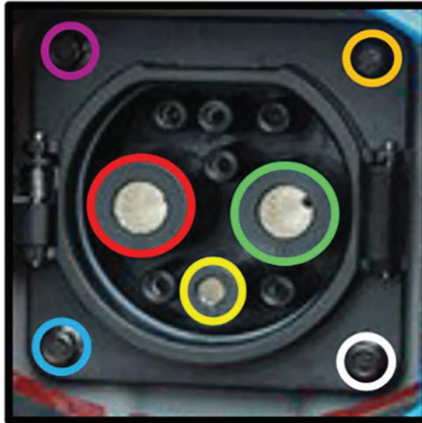
Figure 7: Hough transform circle detection and feature point extraction
