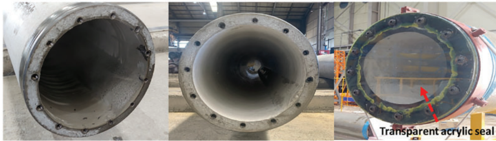
Figure 2: Picture of SFT system experiment model (tunnel body)
