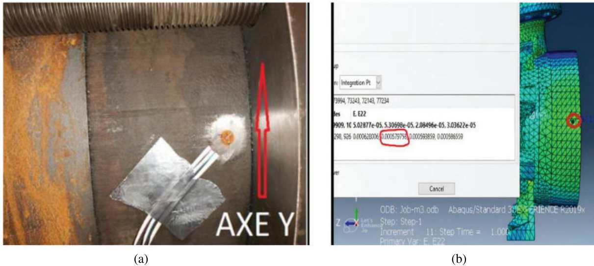
Figure 7: (a) Experimental location of the strain gauge (b) numerical results (pressure = 1500 PSI)
