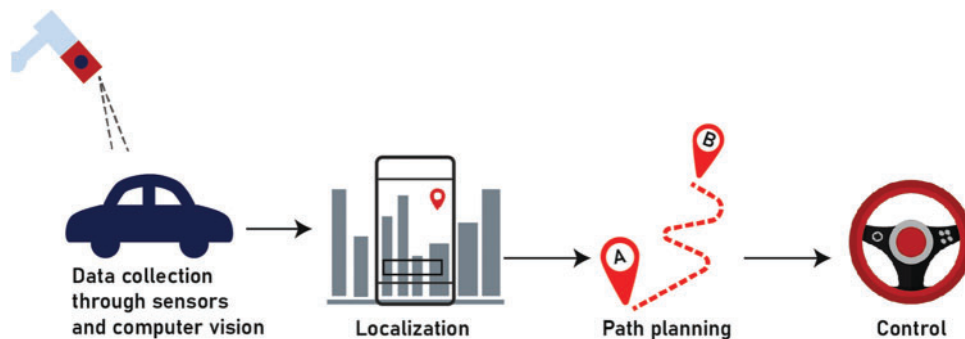
Figure 11: Typical flowchart of DL-based CV in autonomous vehicles
