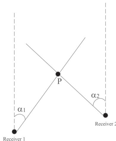
**Figure 7:** AoA schematic diagram
