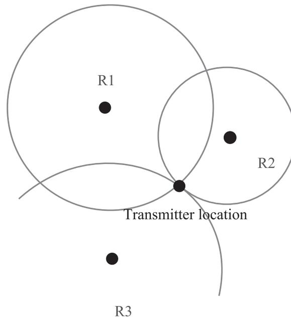
**Figure 6:** TDoA schematic diagram
