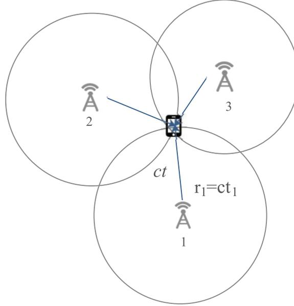
**Figure 5:** ToA schematic diagram
