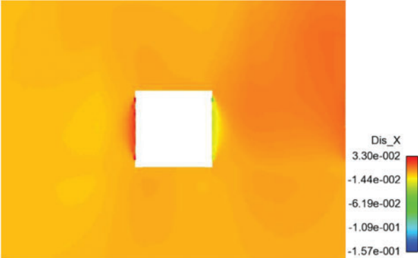
Figure 12: Horizontal displacement of roadway surrounding rock under original support scheme (unit: m)
