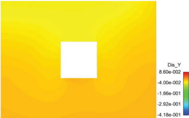
Figure 13: Vertical displacement of roadway surrounding rock under original support scheme (unit: m)
