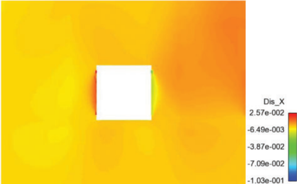
Figure 14: Horizontal displacement of roadway surrounding rock under modified support scheme (unit: m)
