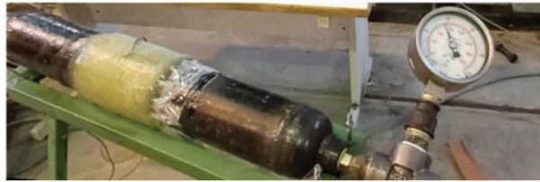
Figure 12: Pipe repaired with Glass Fiber Reinforced Polymer (GFRP) under internal pressure
