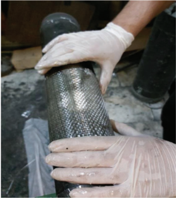
Figure 11: Impregnation of composite layers with resin
