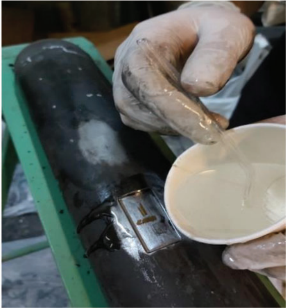
Figure 10: Filling the artificial defect with hardener resin
