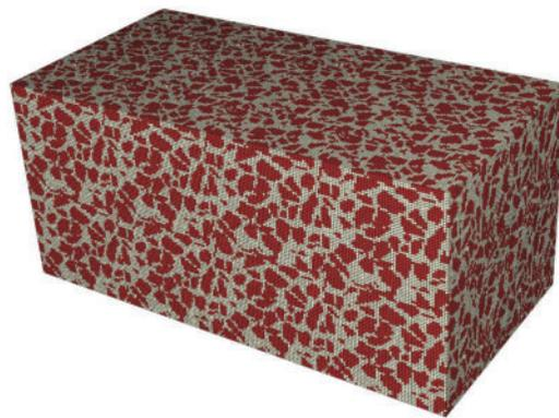
**Figure 19:** FE mesh in reference solution for DNS by Abaqus (1885529 nodes)
