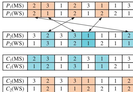
**Figure 6: Multi-point intersection of machines and workers**
