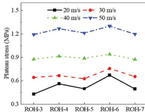
**Figure 16:** Plateau stress of each gradient at different speeds
