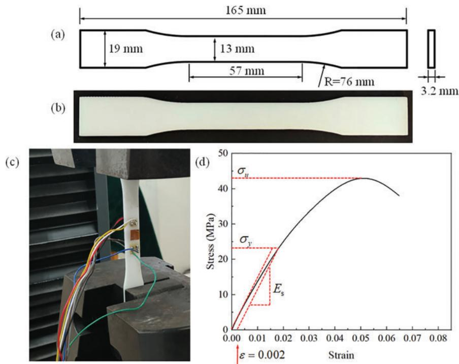
**Figure 4:** (a) Geometric dimensions of dog-bone shaped, (b) standard tensile specimens, (c) perform tensile test setup for standard tensile specimens, and (d) stress-strain curve of C-UV 9400E
