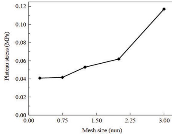
**Figure 3:** Plateau stress of ROH with different mesh sizes
