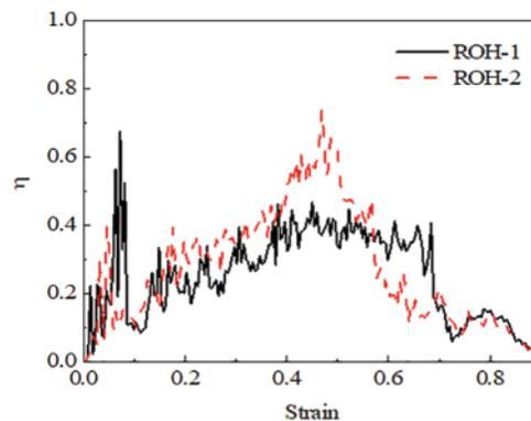
**Figure 12:** Energy absorption efficiency of ROH-1 and ROH-2 under 20 m/s impact
