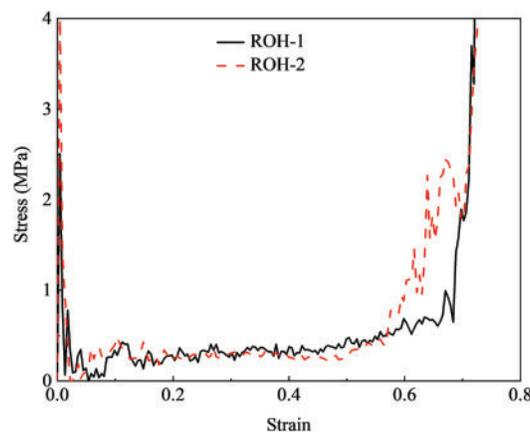
**Figure 10:** Stress-strain curves of ROH-1 and ROH-2 at an impact speed of 20 m/s
