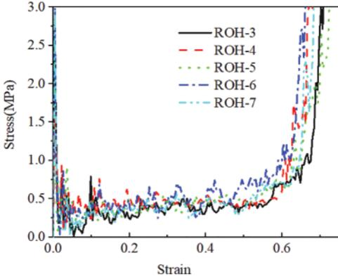
Figure 14: Stress-strain curves of each gradient at an impact speed of 20 m/s
