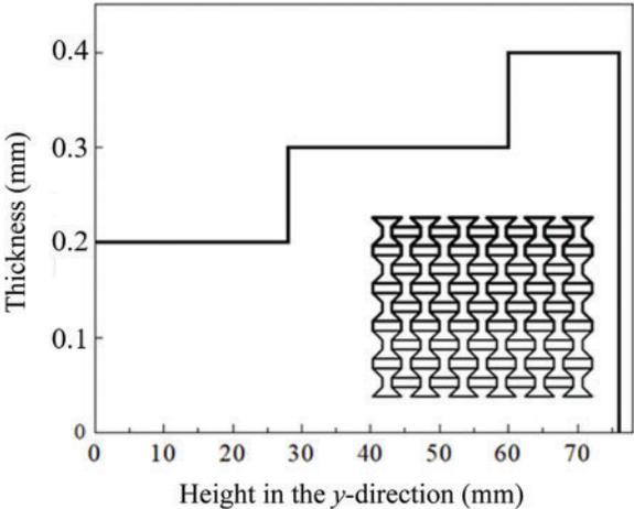
Figure 8: Cell wall thickness of ROH-2
