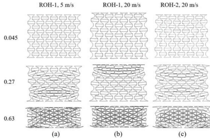
**Figure 9:** Deformation patterns before and after gradient design along the impact direction
