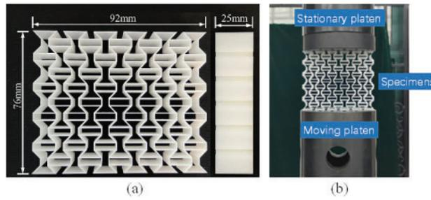
**Figure 5:** (a) Specimens of C-UV 9400E material fabricated by 3D printing and (b) in-plane quasi-static compressive test setup for ROH
