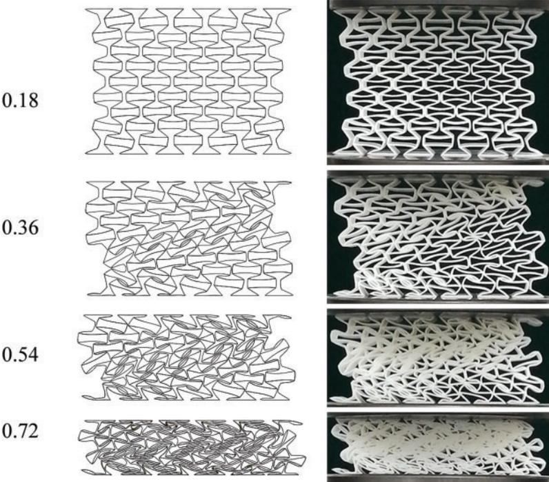
Figure 7: Comparison of deformation modes between experiments and simulations
