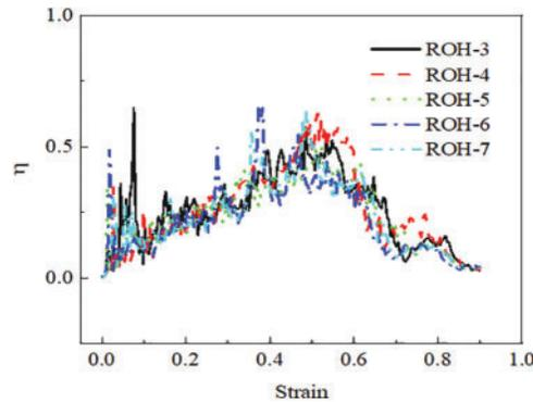
**Figure 15:** Energy absorption efficiency curves of each gradient at an impact speed of 20 m/s
