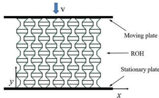
**Figure 2:** Finite element model of ROH under axial compression
