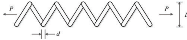
Figure 19: Schematic of tension/compression spring design
