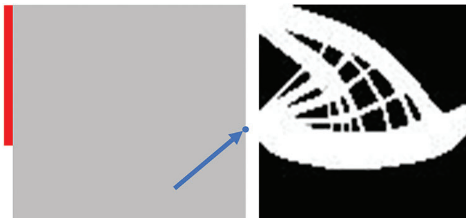
Figure 1: Force/Boundary conditions and corresponding topology optimization structure
