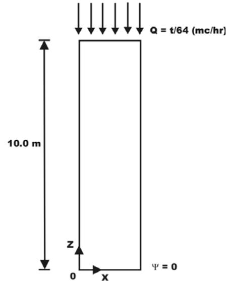
**Figure 1 :** Geometrical setting of variably saturated Test Case 1
