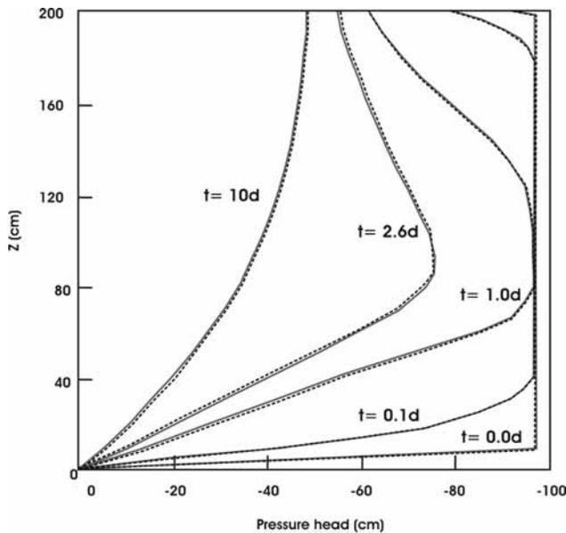
**Figure 6** : Solution for Test Case 3 (Infiltration). CM (solid line) and FEM (dashed line)
