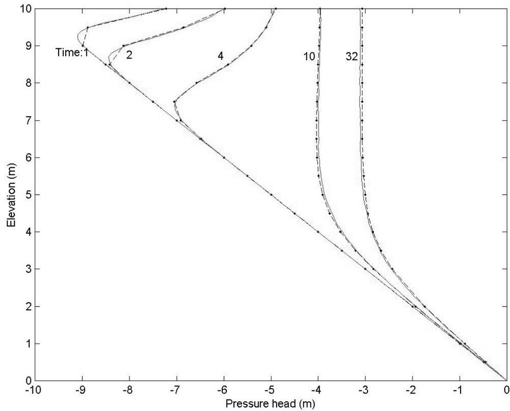
Figure 2 : Pressure Head for Test Case 1. CM (solid line) and FEM (dashed line)
