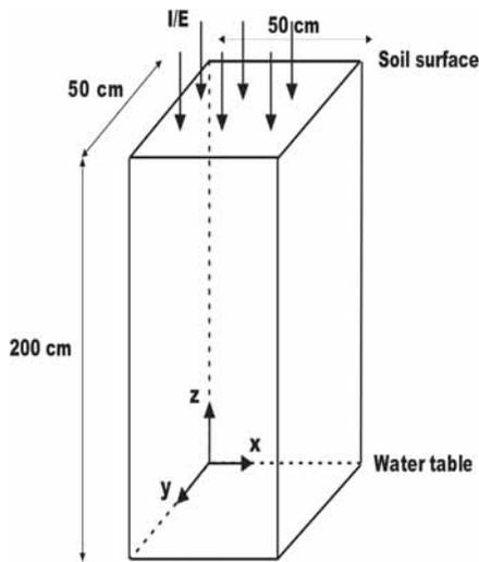
**Figure 5** : Geometrical setting of variably saturated Test Case 3
