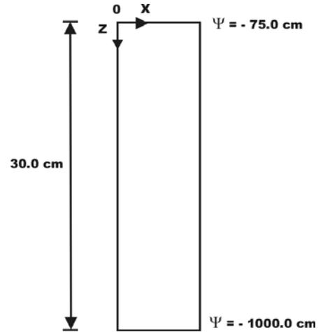
**Figure 3 :** Geometrical setting of variably saturated Test Case 2
