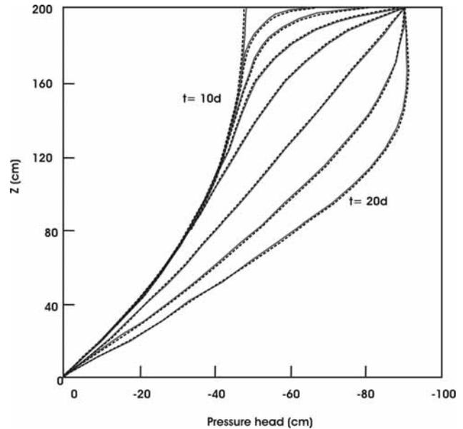
**Figure 7** : Solution for Test Case 3 (Evaporation). CM (solid line) and FEM (dashed line)
