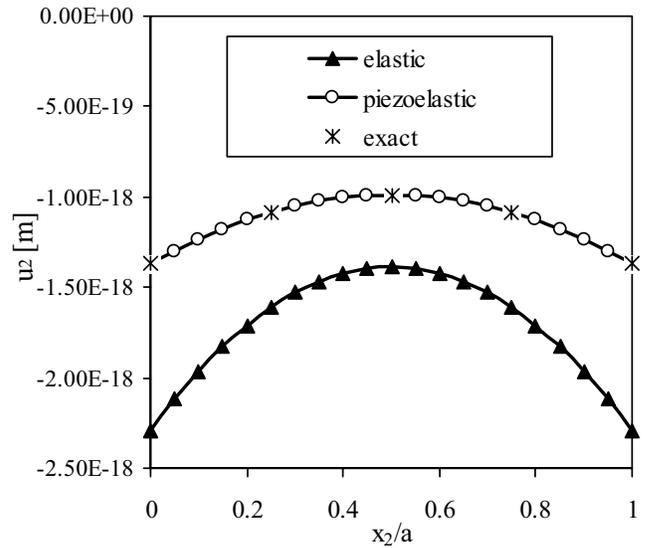
Figure 3 : Variation of the mechanical displacement  $u_2$  with normalized coordinate  $x_2/a$
