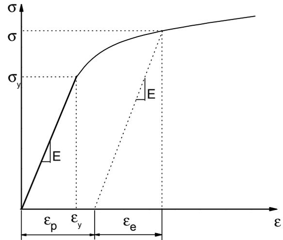
Figure 1: A schematic of power law material model
