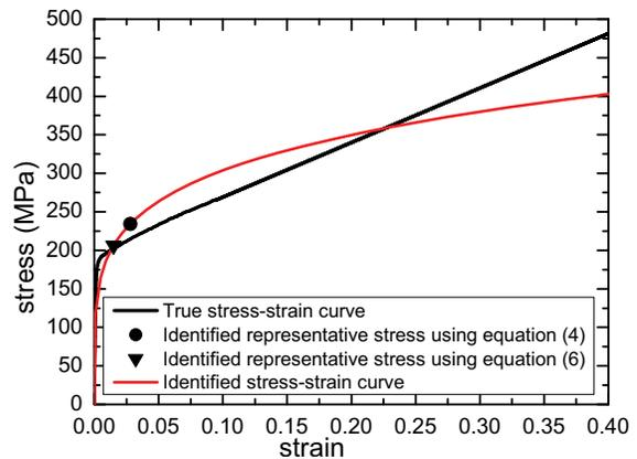
Figure 5: Comparison of the identified stress-strain curve with the real one
