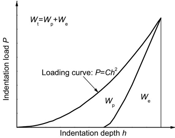
Figure 2: A schematic of the indentation loading curvature  $C$ , reversible work  $W_e$  and total work  $W_t$
