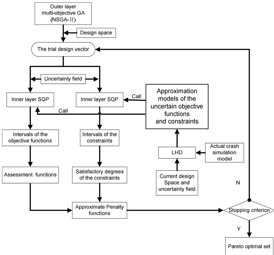
Figure 1: Nesting optimization based on the approximation models
