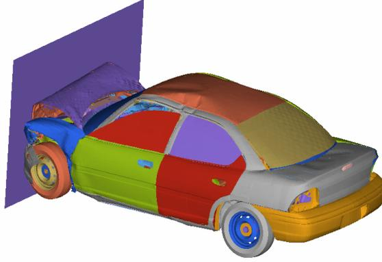
Figure 6: The deformation of the full frontal impact
