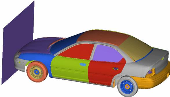
Figure 5: Finite element model of vehicle
