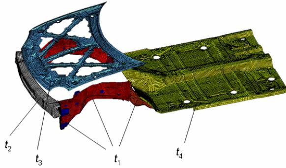
Figure 2: Design variables of the vehicle model
