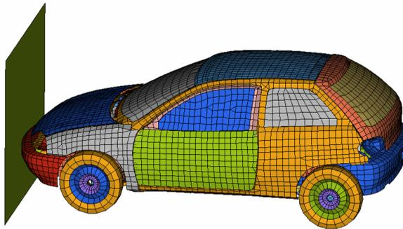
Figure 12: The finite element model of the vehicle
