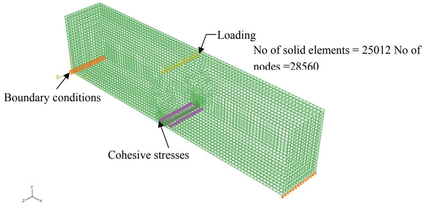
Figure 7: FE mesh (crack length=4mm)
