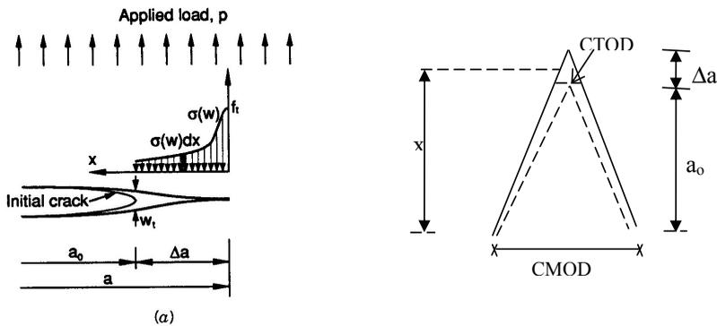
**(a) Modelling of quasi-brittle crack with crack surfaces in contact**
