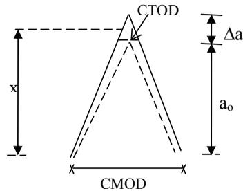
(b) Schematic diagram of crack Opening displacement
