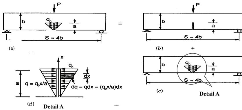
Figure 3: Illustration of superposition principle
