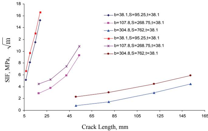
Figure 13: Crack length vs SIF for geometrically similar components
