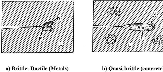
Figure 1: FPZ in ductile and brittle materials
