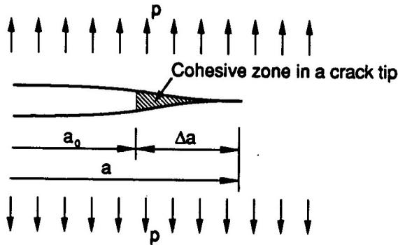
Figure 2: Mode I crack for fictitious crack approach
