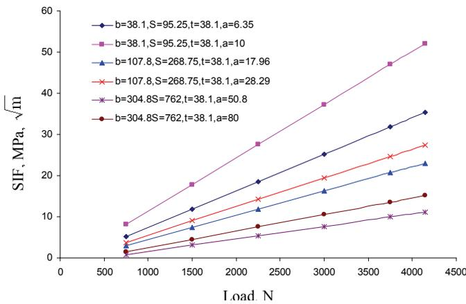
Figure 14: Load vs SIF for geometrically similar components
