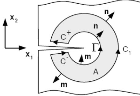
Figure 5: Closed contour  $C = C_1 - \Gamma + C^+ + C^-$  enclosing a simply connected region A
