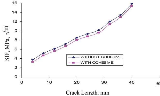
Figure 12: Crack length vs SIF
