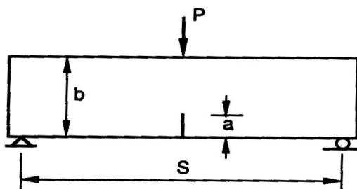
Figure 6: Geometry of 3 point bending specimen
