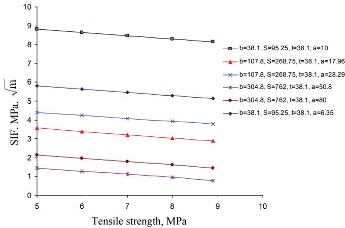
Figure 15: Tensile strength vs SIF for geometrically similar components
