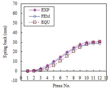
Figure 14: Spring back at each press position
