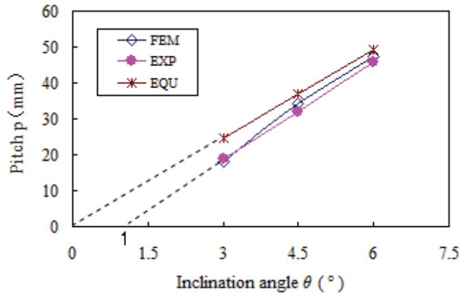
Figure 18: Relationship between inclination angle of the punch and the spiral pitch
