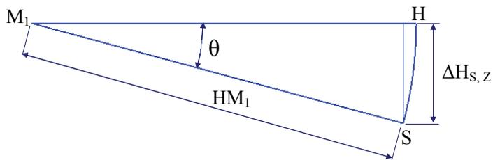
Figure 7: Displacement of point S in Z axial direction
