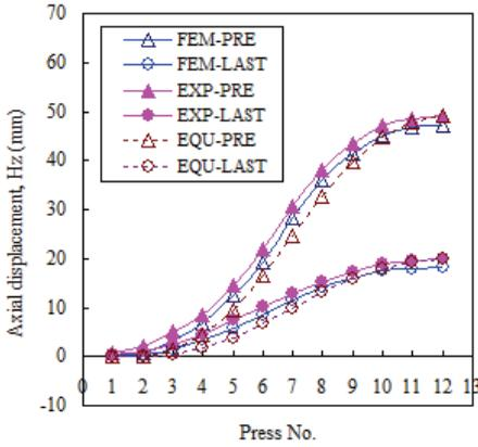
Figure 13: Opening distance before and after spring back at each press position
