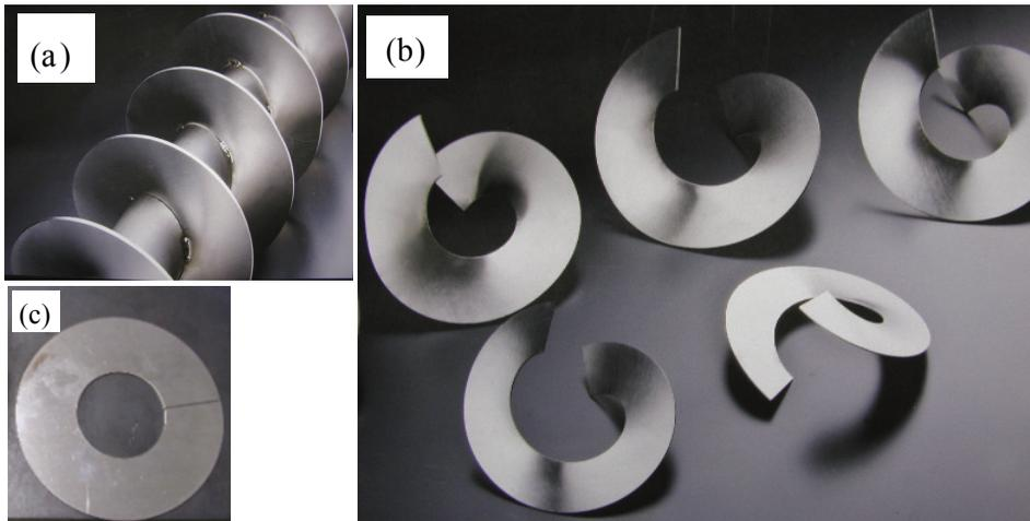
Figure 1: Specimens: screw (a), spiral plates (b) and disk with a hole and a slit (c)
