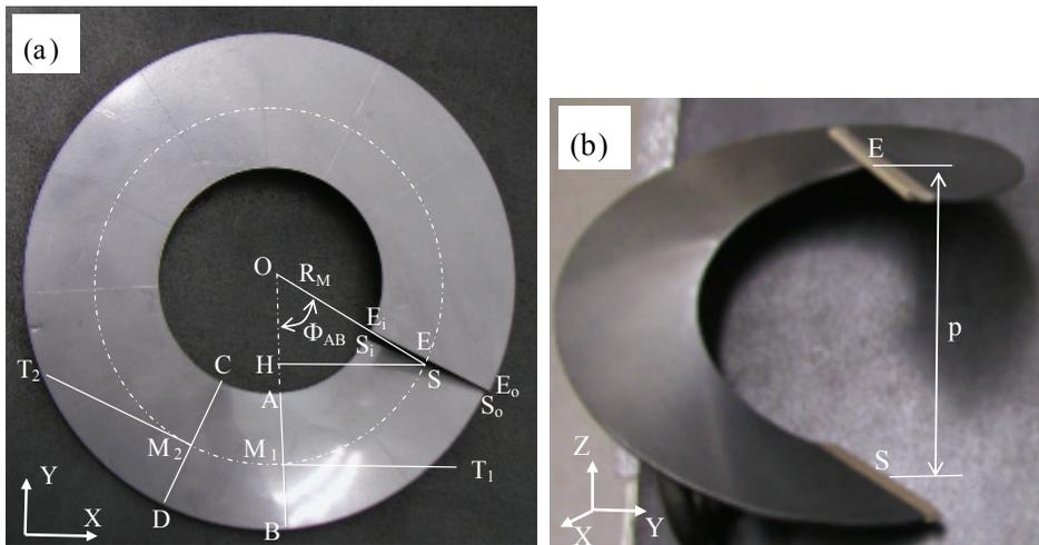
Figure 6: Deformation of the disk at the third press (a) and the last press (b)
