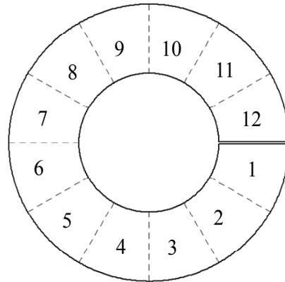
Figure 5: A sequence of positions for press operations
