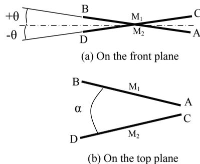
Figure 3: Angles formed by the punches and dies on the front plane (a) and top plane (b)
