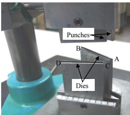
Figure 2: A pair of punches and dies
