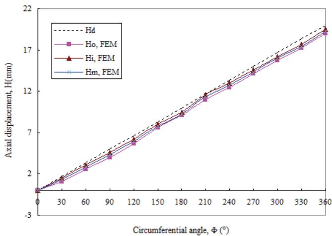
Figure 16: Relationship between circumferential angle (press position) and axial displacement of the spiral plate —FEM simulation
