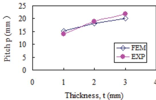
Figure 17: Relationship between thickness of specimen and spiral pitch
