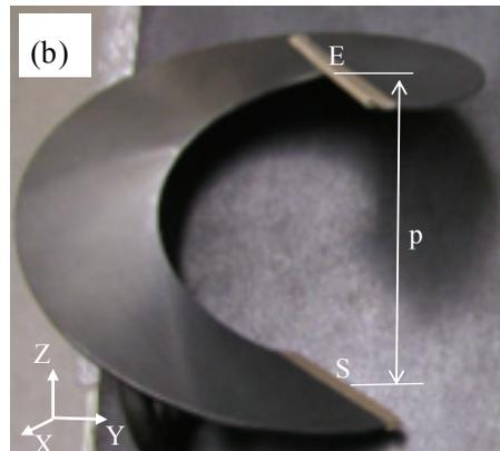
Figure 6: Deformation of the disk at the third press (a) and the last press (b)
