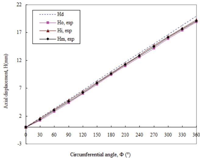
Figure 15: Relationship between circumferential angle (press position) and axial displacement of the spiral plate —experiment
