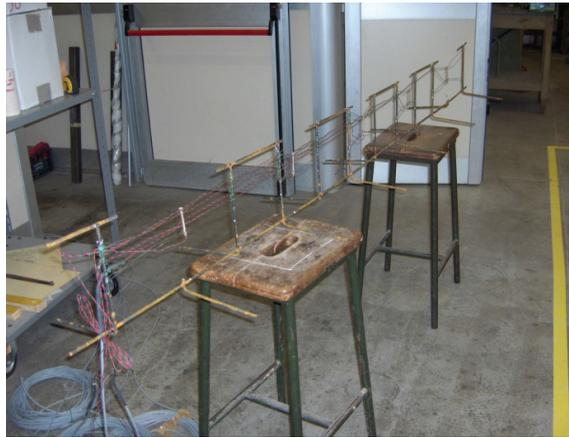
Figure 17: Positioning of the strain gauges over the metallic support
