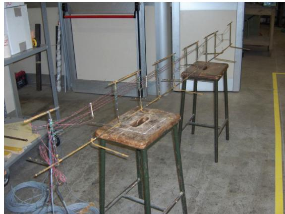
Figure 17: Positioning of the strain gauges over the metallic support
