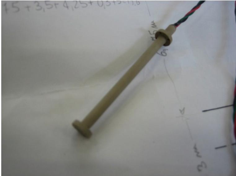
Figure 15: Luchsinger strain-gauge for embedment in concrete
