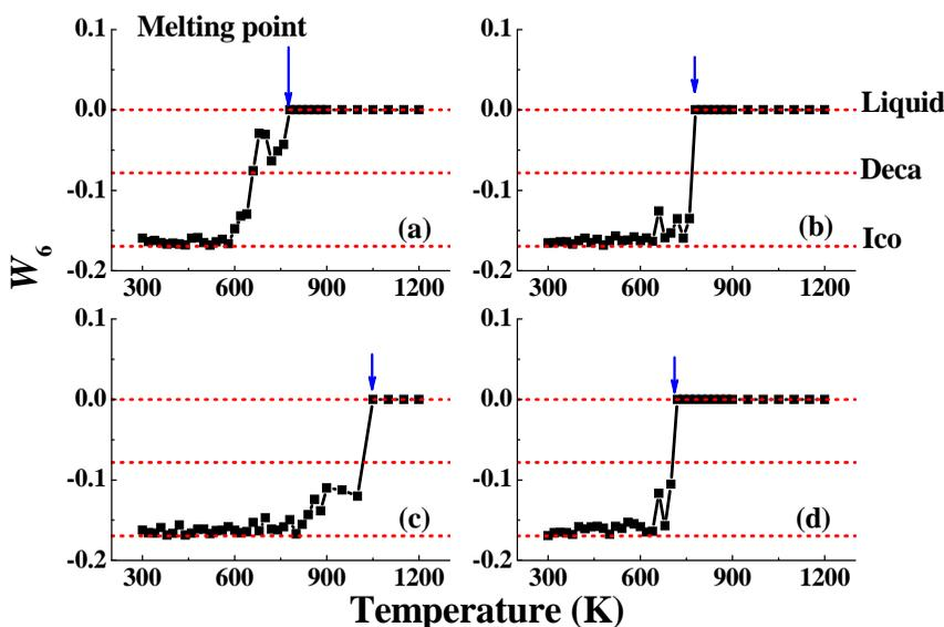
Figure 3: Variation of  $W_6$  for the mixed (a) and core-shell  $(\text{PdAg})_{309}$  (b),  $\text{Pd}_{309}$  (c), and  $\text{Ag}_{309}$  (d) with temperature.
