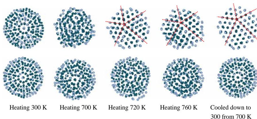
Figure 4: Snapshots of the mixed (top) and core-shell (bottom)  $(\text{PdAg})_{309}$  at different temperatures
