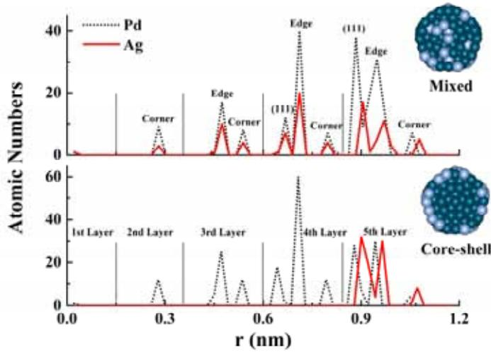
Figure 1: Atomic number along the radius direction for the mixed and core-shell  $(\text{PdAg})_{309}$  after the cluster relaxed for 0.5 ns at 300 K. The sphere is the cross section of the cluster. The Pd atom is represented by dark blue and the Ag atom by light blue
