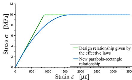
Figure 49: Comparison between the new parabola-rectangle relationship and the design relationship given by the effective laws
