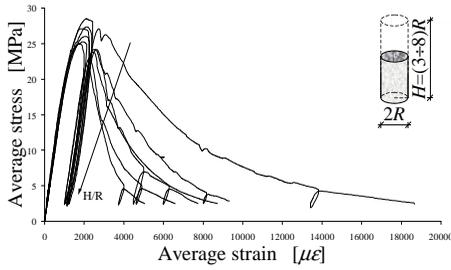
Figure 10: Size effect for the average stress-average strain diagrams
