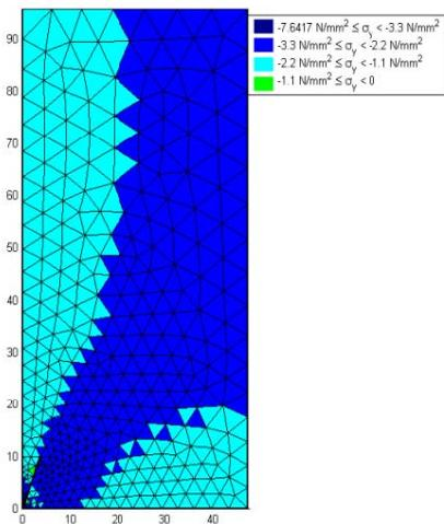
Figure 18: Axial stress analysis on the longitudinal section for plain concrete
