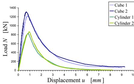
Figure 37: Load-displacement diagrams for Mixture 1
