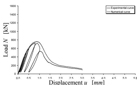
Figure 21: Numerical and experimental results for the unwrapped specimens
