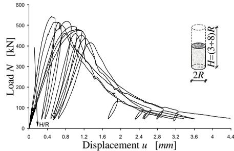
Figure 9: Size effect for the load-displacement diagrams
