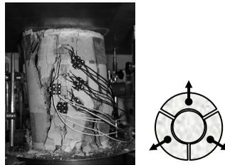
Figure 1: Vertical cracks on the surface of a concrete specimen originated by the splitting of incoherent material isolated by the propagation of internal macro-cracks
