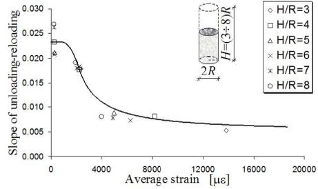
Figure 11: Interpolating law of the average slope of the unloading-reloading cycles
