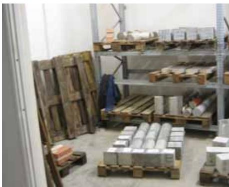
Figure 31: Curing room under controlled thermo-hygrometric conditions
