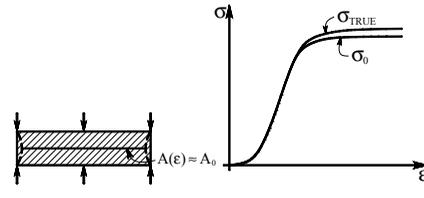
Figure 26: Effect of stress definition on the shape of the stress-strain curve for small  $H/(2R)$  ratio [Hudson Brown and Fairhurst (1971)]
