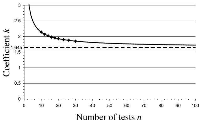
Figure 45: Interpolation of the coefficient  $k$  (90% confidence degree)
