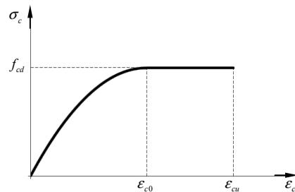
Figure 44: Design stress-strain diagram for concrete
