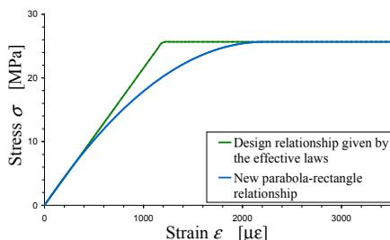
Figure 47: Comparison between the new parabola-rectangle relationship and the design relationship given by the effective laws
