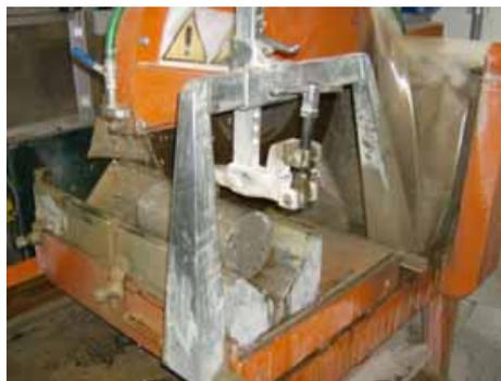
Figure 32: Automatic cylinder-end grinder
