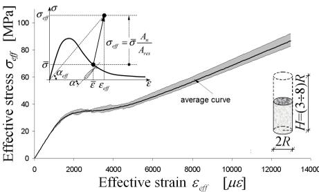
Figure 12:  $\sigma_{eff} - \epsilon_{eff}$  dispersion range for variable slenderness and average curve
