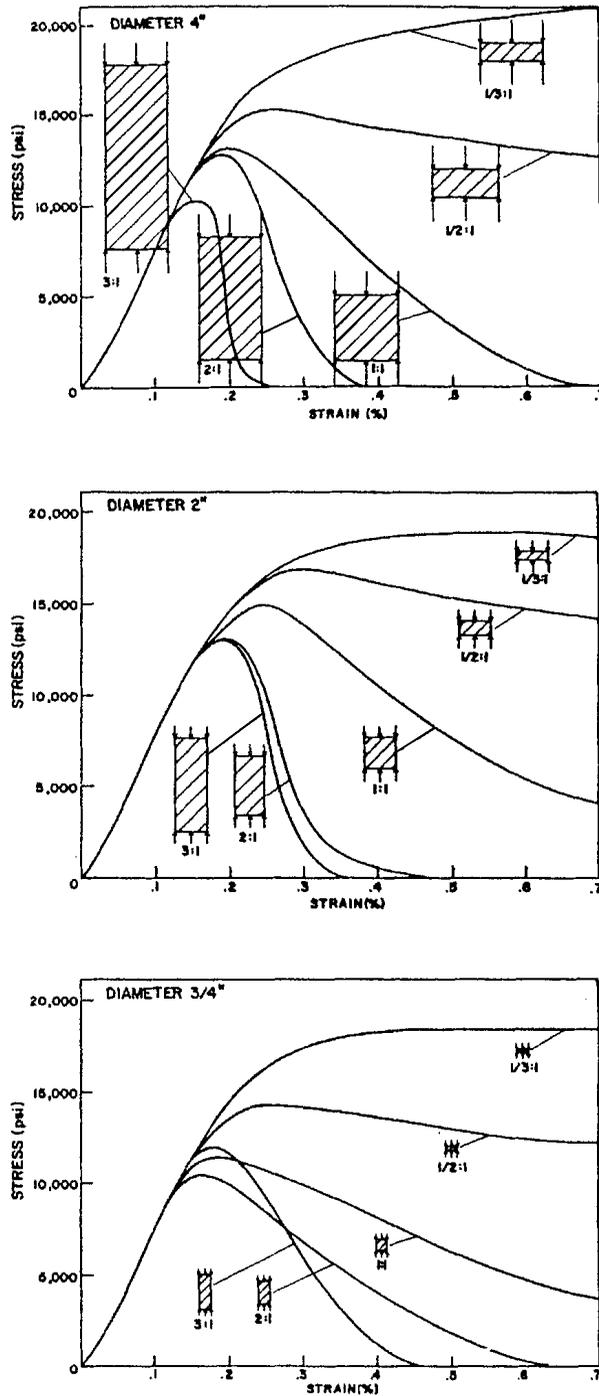
Figure 24: Influence of specimen shape on the  $\bar{\sigma} - \bar{\epsilon}$  curve for marble loaded in uniaxial compression [Hudson Brown and Fairhurst (1971)]
