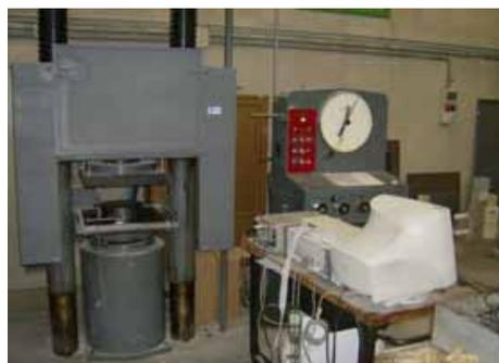
Figure 36: Compression-testing machine and acquisition apparatus
