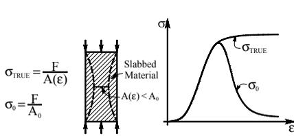
Figure 25: Effect of stress definition on the shape of the stress-strain curve for large  $H/(2R)$  ratio [Hudson Brown and Fairhurst (1971)]
