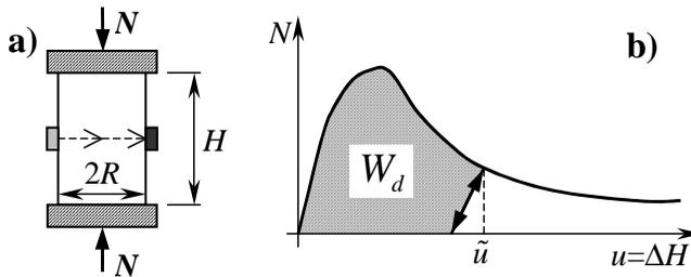
Figure 5: a) Test set-up for the acquisition of  $D_1$ ; b) Evaluation of  $W_d$  for the acquisition of  $D_2$
