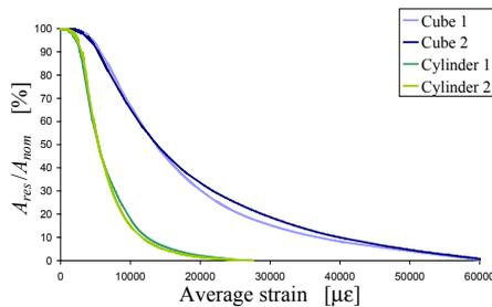
Figure 39: Shape-effect on the decrease of resistant area for Mixture 1
