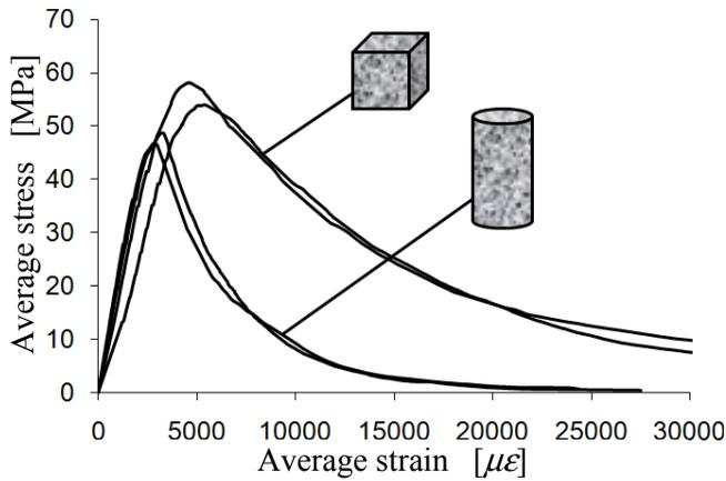
Figure 27: Shape-effect for cubic and cylindrical concrete specimens
