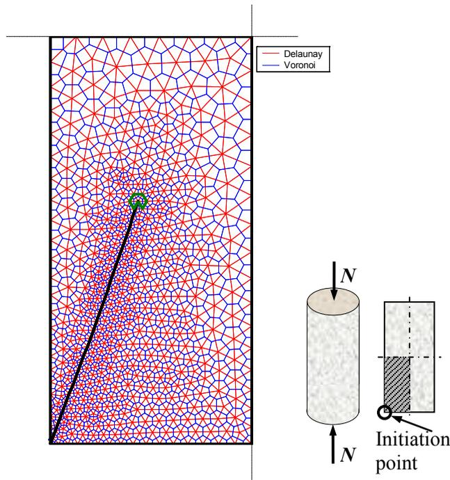
Figure 16: Crack path for the bottom-left quarter of the longitudinal section
