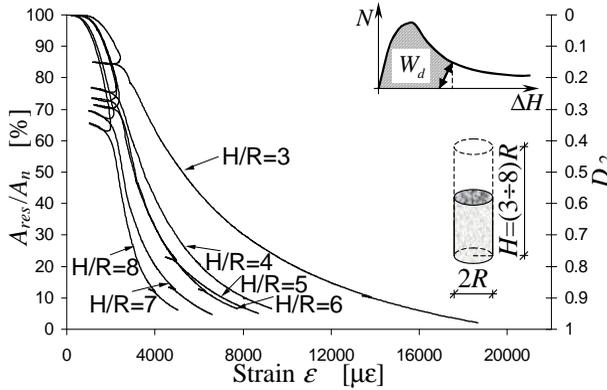
Figure 7: Normalized resistant area and  $D_2$  damage law for variable slenderness
