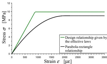
Figure 48: Comparison between the parabola-rectangle relationship and the design relationship given by the effective laws
