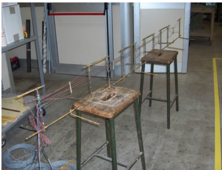
Figure 10: Positioning of the strain gauges over the metallic support
