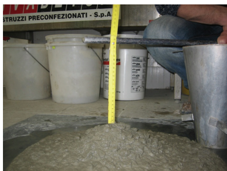
Figure 15: Assessment of the fresh concrete workability by means of the Abrams slump test
