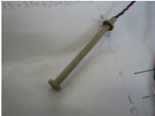
Figure 8: Luchsinger strain-gauge for embedment in concrete
