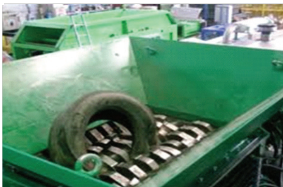
Figure 1: Grinding of the tire tread
