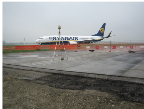
Figure 11: Base station receiver for GPS topographic surveying positioned on the centerline at the end of the experimental segment
