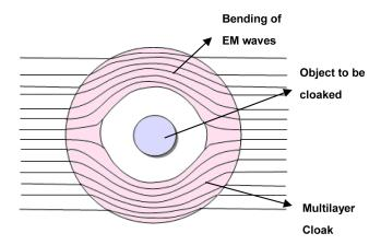
Figure 1: Illustration of cylindrical cloak.
