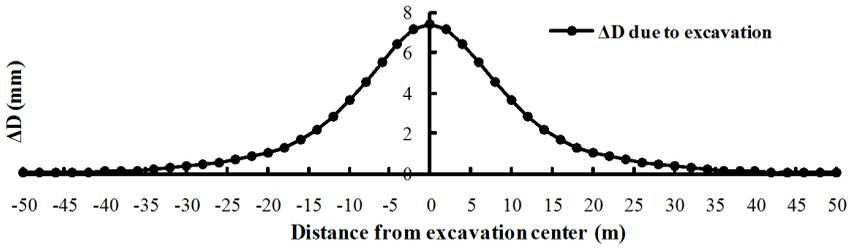
Figure 11: Cross section deformation of tunnel lining
