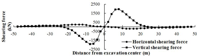
Figure 13: Shearing forces between tunnel rings
