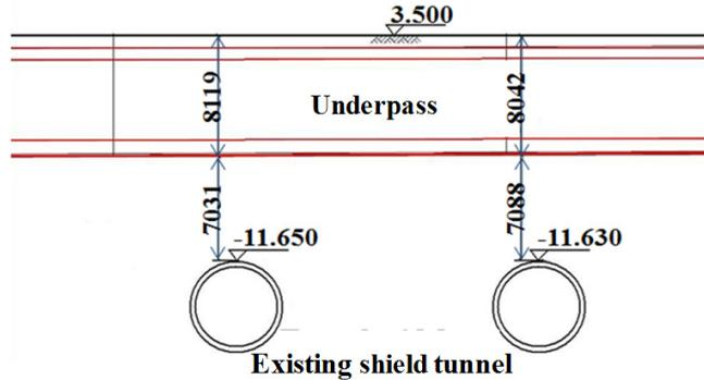
Figure 1: Underpass and the existing shield tunnel (Unit: mm for distance, m for elevation)
