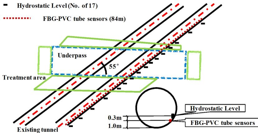
Figure 2: Site plane and layout of the instrumentation
