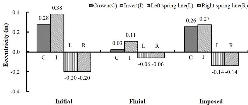
Figure 17: Eccentricity of tunnel lining below the excavation center
