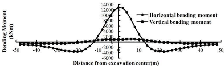
Figure 14: Bending moment along the tunnel
