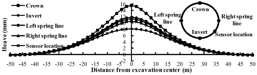
Figure 10: Tunnel heave along longitudinal direction of tunnel at different circumferential locations
