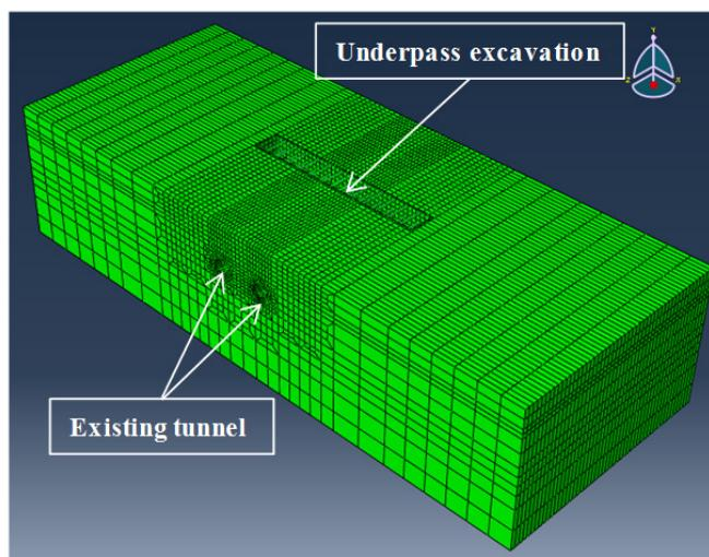
Figure 7: Mesh of the 3D FE model
