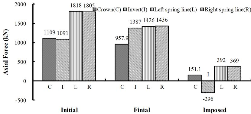
Figure 16: Axial force of tunnel lining under the excavation center
