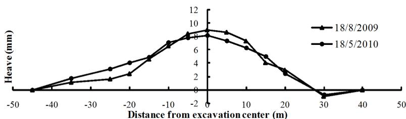
Figure 6: Tunnel heave measured by Hydrostatic Level
