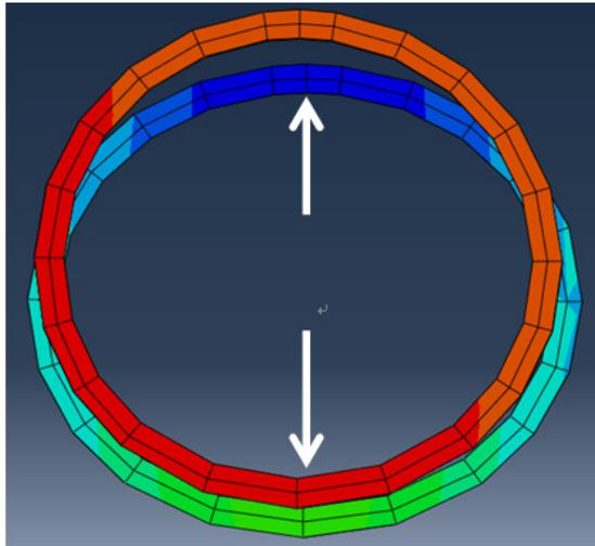
Figure 12: Joint movement due to the nonuniform cross section deformation of tunnel rings
