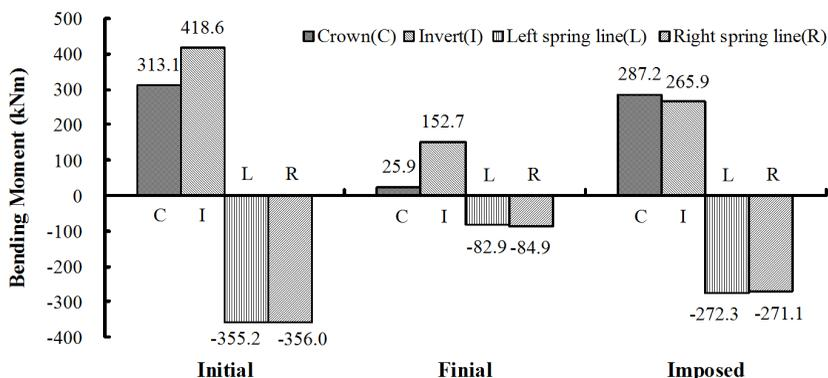
Figure 15: Bending moment of tunnel lining below the excavation center
