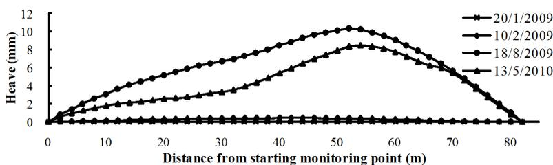
Figure 5: Tunnel heave measured by FBG-PVC tube sensor
