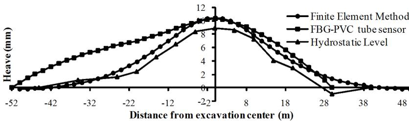
Figure 9: Comparison of tunnel heaves by FEM, FBG-PVC tube sensor and Hydrostatic Level when the excavation was completed
