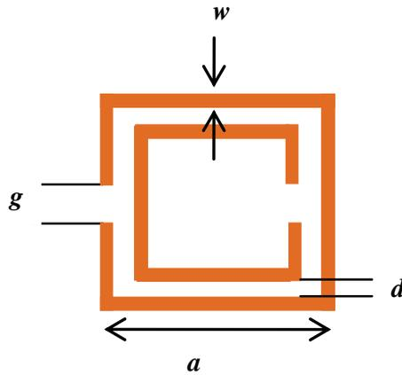
Figure 1: Schematic of a square split ring resonator.
