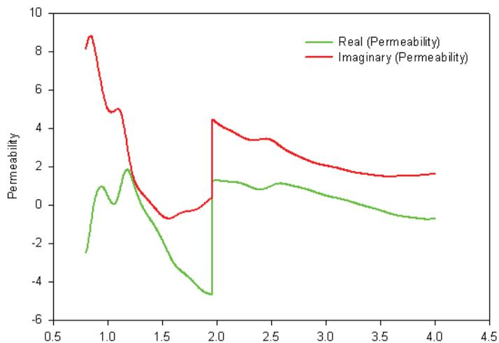
Figure 5: Extracted permeability of the designed square SRR.
