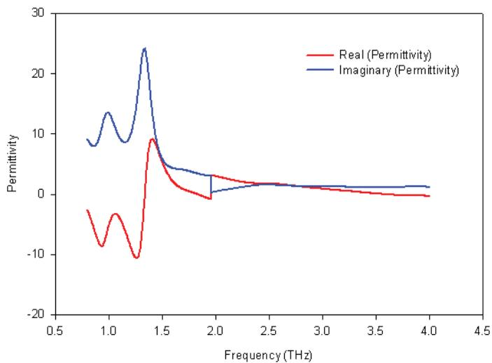
Figure 4: Extracted permittivity of the designed square SRR.
