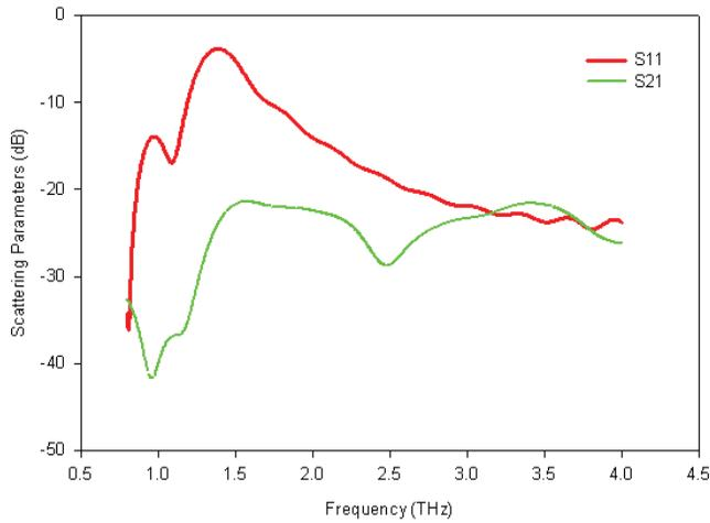
Figure 3: Scattering parameters  $S_{11}$  and  $S_{21}$  parameters of the designed square SRR optimized using PSO algorithm.
