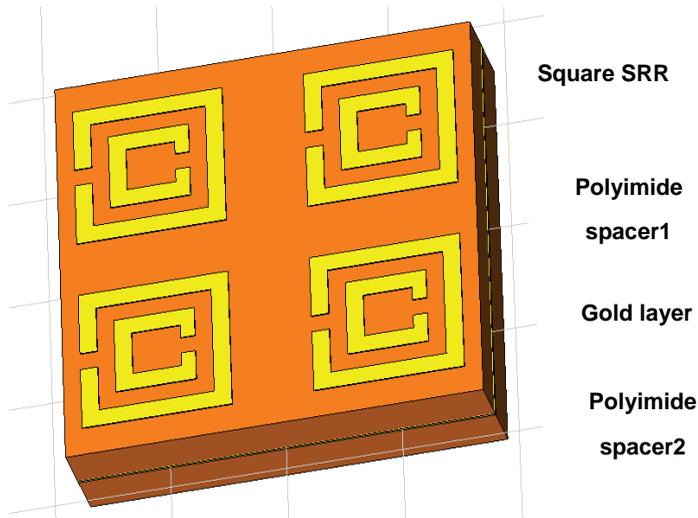
Figure 6: The four layer Metamaterial RAM design. The top layer consists of four optimized square SRR structures
