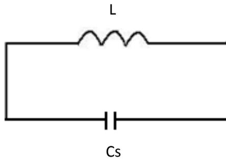
Figure 2: Equivalent circuit of the square SRR
