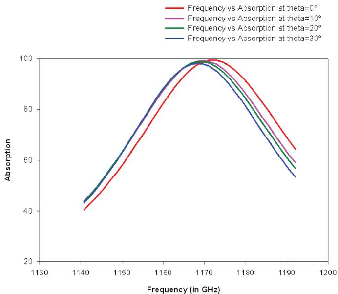
Figure 7: Absorption characteristics of the RAM (absorber) designed by soft computing PSO algorithm.
