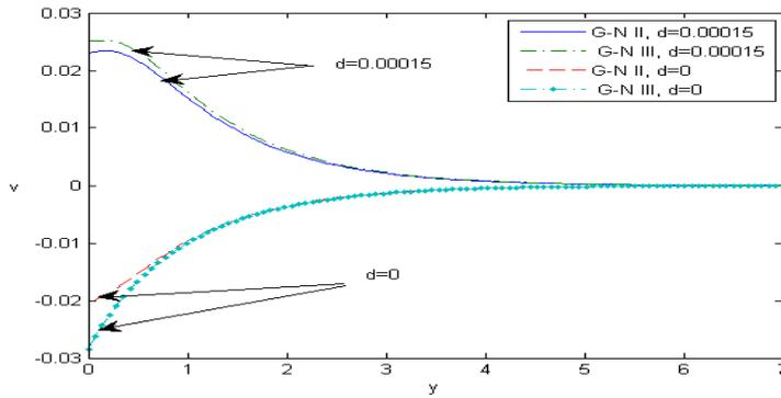
Figure 14: The displacement component  $v$  distribution against  $y$  with and without two temperature.
