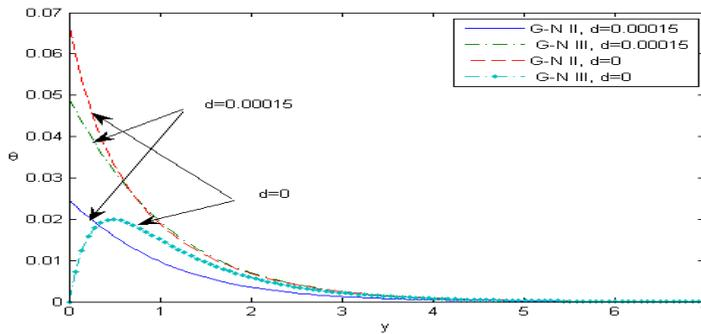
Figure 15: The distribution of the conductive temperature  $\theta$  against  $y$  with and without two temperature.
