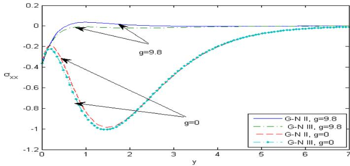
Figure 4: The distribution of the stress tensor component  $\sigma_{xx}$  against  $y$  with and without gravity.
