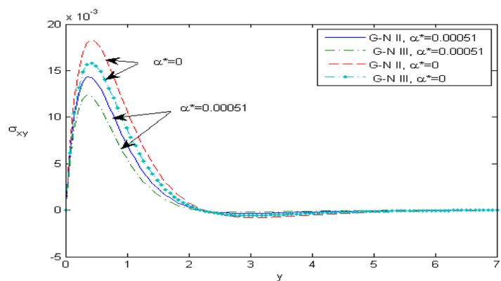
Figure 11: The distribution of the stress tensor  $\sigma_{xy}$  against  $y$  with and without temperature dependent.
