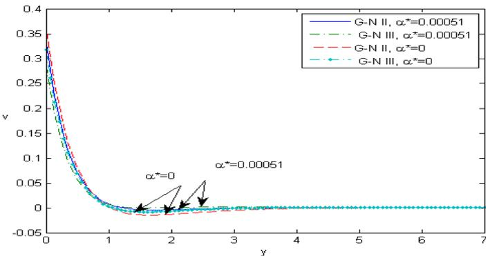
Figure 8: The displacement component  $v$  distribution against  $y$  with and without temperature dependent.
