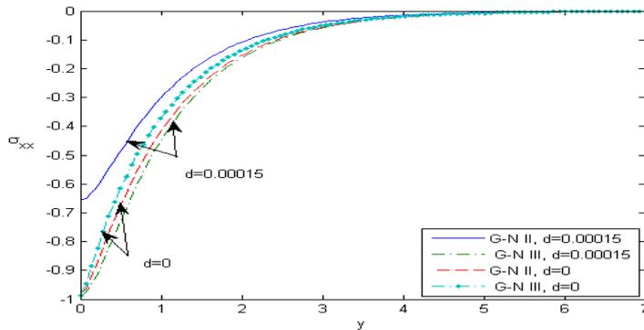
Figure 16: The distribution of the stress tensor component  $\sigma_{xx}$  against  $y$  with and without two temperature.
