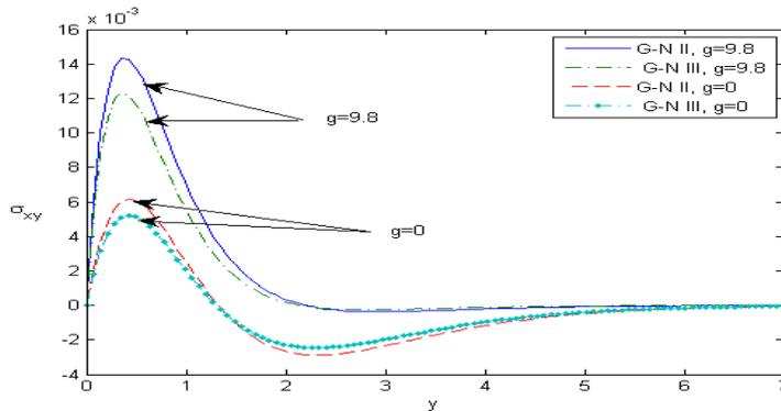
Figure 5: The distribution of the stress tensor component  $\sigma_{xy}$  against  $y$  with and without gravity.
