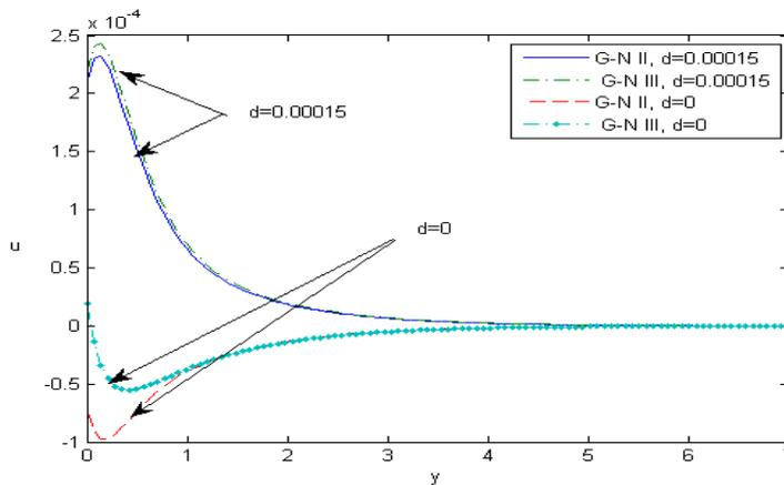
Figure 13: The displacement component  $u$  distribution against  $y$  with and without two temperature.
