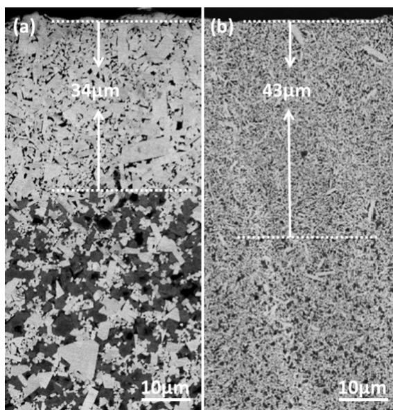
Figure 3: Microstructure at the surface of cemented carbide prepared by gradient sintering after (a) vacuum pre-sintering and (b) low pressure pre-sintering.
