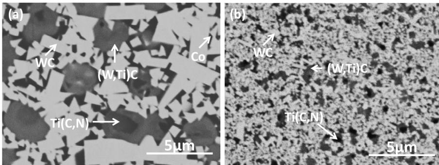
Figure 1: The microstructure of carbide cemented after (a) vacuum pre-sintering and (b) low pressure pre-sintering.
