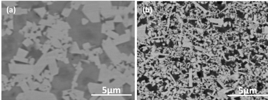
Figure 4: The inside microstructure of carbide cemented prepared by gradient sintering after (a) vacuum pre-sintering and (b) low pressure pre-sintering.
