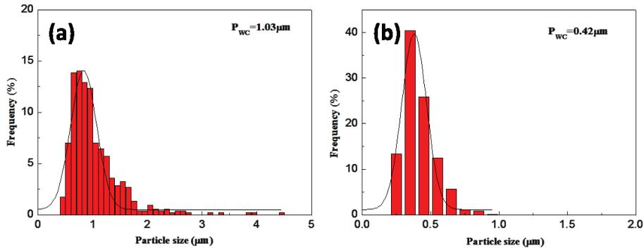
Figure 5: Distribution of WC grain size in the alloys prepared by gradient sintering after (a) vacuum pre-sintering and (b) low pressure pre-sintering.
