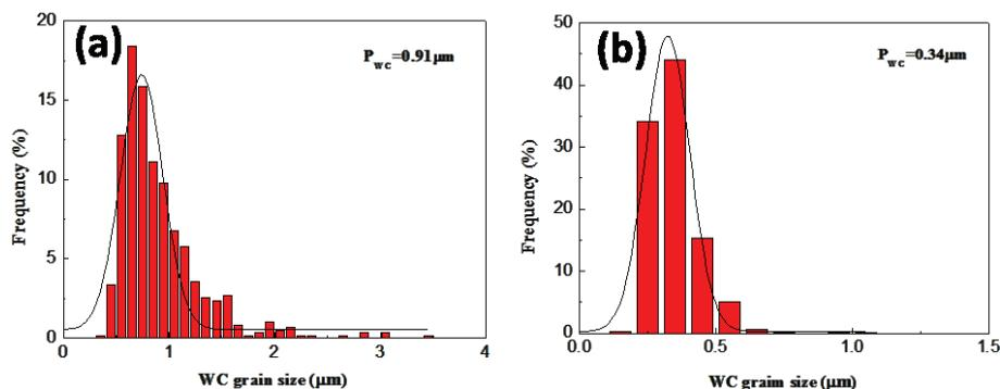
Figure 2: The WC grain size distributions of specimens prepared by (a) vacuum pre-sintering and (b) low pressure pre-sintering.
