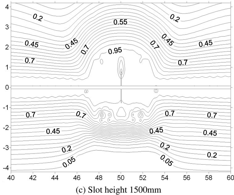
Figure 4: Damage distribution of coal seam of sectional view  $\alpha$  under different slot heights (coordinate axis unit: m).
