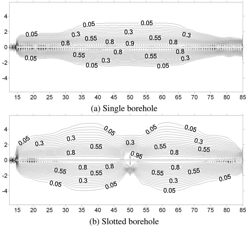
Figure 2: Damage distribution of coal seam of sectional view  $\alpha$  (coordinate axis unit: m)
