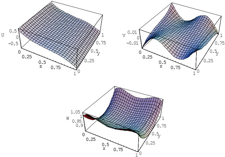
Figure 6: Displacement profiles of the first mode for the sinusoidally graded square rod at  $kd = 3$ .
