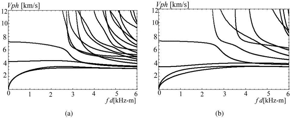
Figure 3: Phase velocity dispersion curves for linearly graded rectangular rods: (a)  $d/h = 1$ , (b)  $d/h = 2$ .
