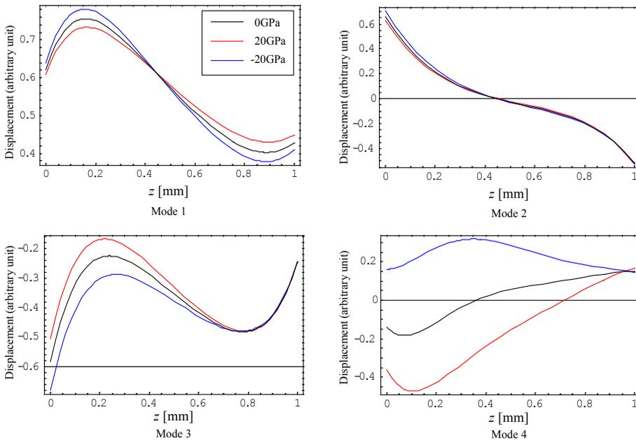
Figure 12:  $u$  displacement distributions at  $y = 0$  for the first four modes of the linearly graded square rod with initial stress.
