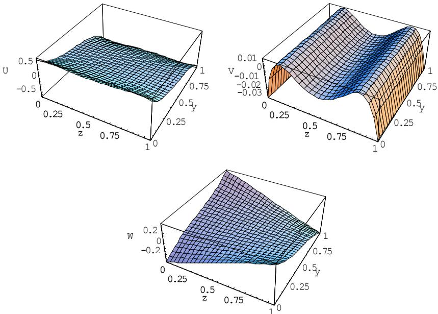
Figure 7: Displacement profiles of the second mode for the sinusoidally graded square rod at  $kd = 3$ .
