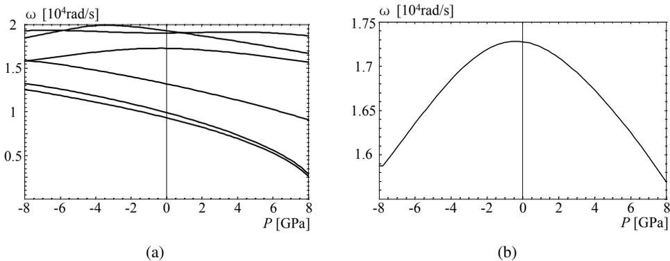
Figure 11: Variation of the frequency with respect to initial stress for the linearly graded square rods: (a) at  $kh = 3$ ; (b) the fourth order mode at  $kh = 3$ .
