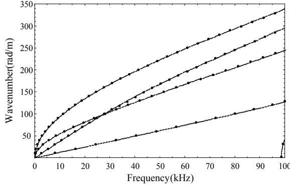
Figure 2: Dispersion curves for a rectangular aluminum rod; lines: Philip W. Loveday’s results, dotted lines: the authors’ results.
