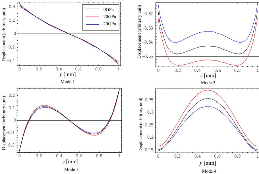
Figure 13:  $u$  displacement distributions at  $z = 0$  for the first four modes of the linearly graded square rod with initial stress.
