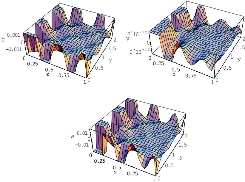
Figure 8: Displacement profiles of the second mode for the linearly graded rectangular rod with  $d/h = 2$  at  $kd = 6000$ .
