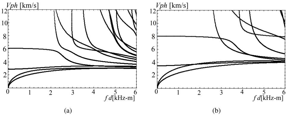
Figure 4: Phase velocity dispersion curves for graded rectangular rods with  $d/h = 2$ : (a) cubically graded rod, (b) sinusoidally graded rod.
