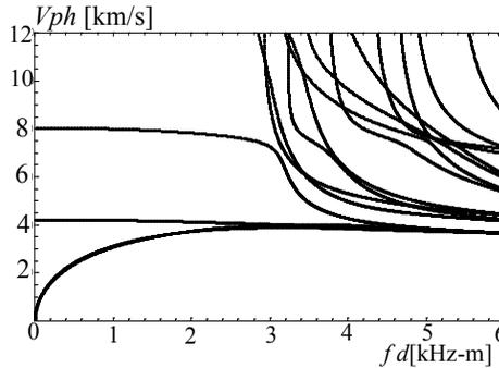
Figure 5: Phase velocity dispersion curves for the sinusoidally graded square rod.
