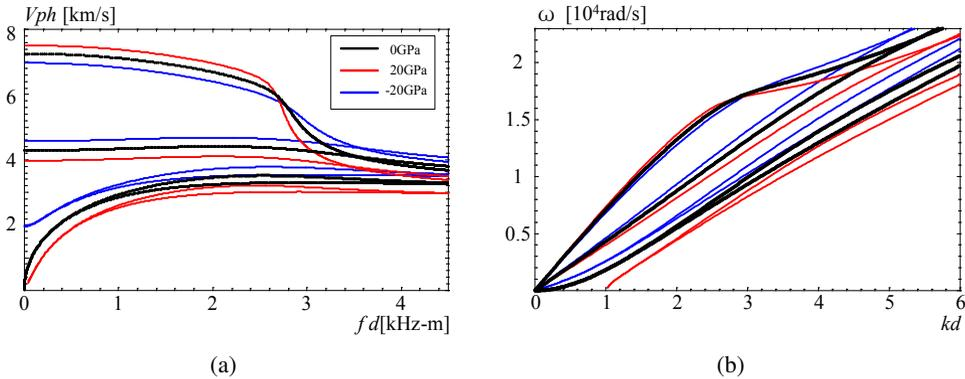
Figure 10: Dispersion curves for the linearly graded square rods with initial stress: (a) frequency spectra; (b) phase velocity spectra.
