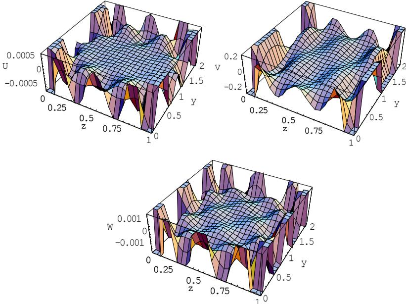
Figure 9: Displacement profiles of the second mode for the sinusoidally graded rectangular rod with  $d/h = 2$  at  $kd = 6000$ .
