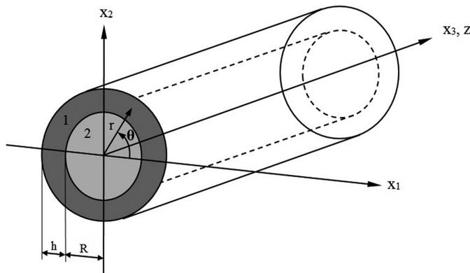
Figure 1: The geometry of the bi-material circular compound cylinder.
