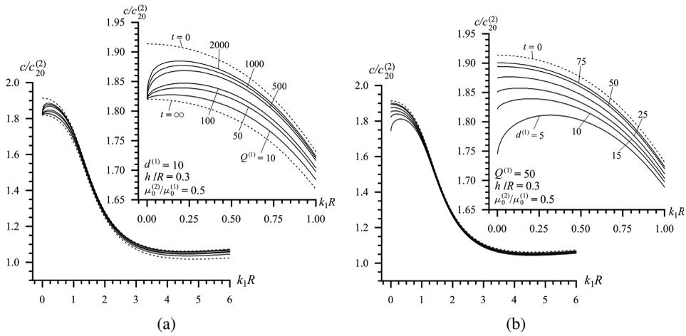
Figure 14: Dispersion curves obtained in the case considered in Fig. 13 under  $h/R = 0.3$ .
