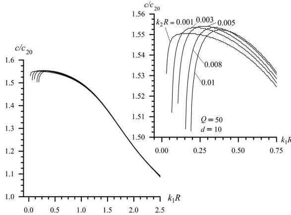
Figure 6: The influence of  $k_2R$  on the cut off values of  $(k_1R)_{c.f.}$  obtained for the non-dispersive attenuation case for the homogeneous solid cylinder under  $Q = 50$  and  $d = 10$ .
