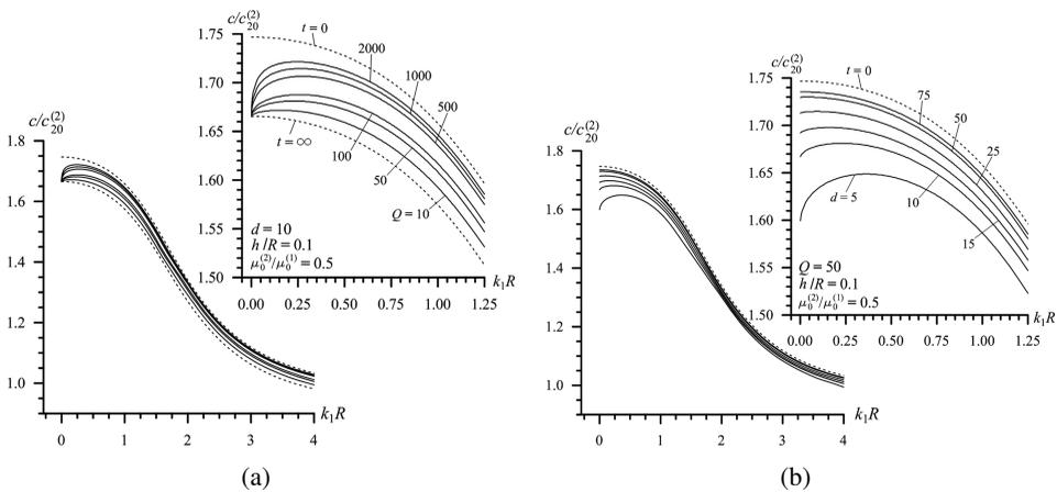
Figure 7: Dispersion curves obtained for various values of the parameter  $Q$  under a fixed value of the parameter  $d (= 10)$  (a) and for various values of the parameter  $d$  under a fixed value of the parameter  $Q (= 50)$  (b) in the V.V. case under  $\mu_0^{(2)}/\mu_0^{(1)} = 0.5$  and  $h/R = 0.1$ .
