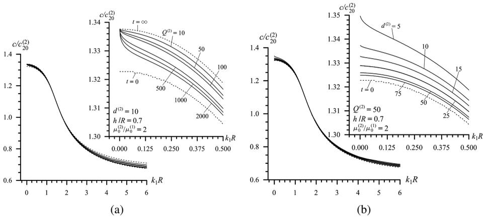
Figure 25: Dispersion curves obtained in the case considered in Fig. 23 under  $h/R = 0.7$ .
