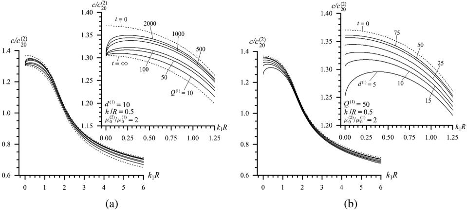
Figure 18: Dispersion curves obtained in the case considered in Fig. 16 under  $h/R = 0.5$ .
