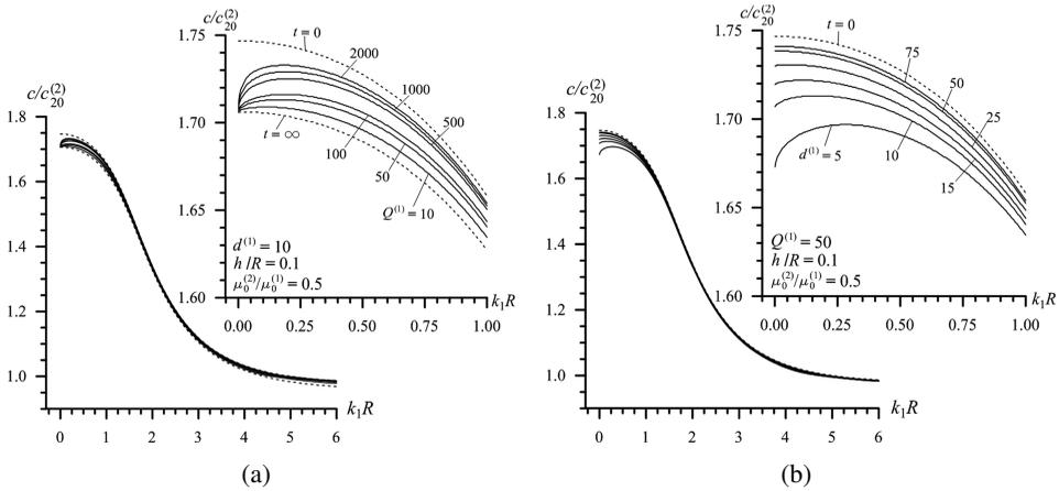
Figure 13: Dispersion curves obtained for various values of the parameter  $Q^{(1)}$  under a fixed value of the parameter  $d^{(1)} (= 10)$  (a) and for various values of the parameter  $d^{(1)}$  under a fixed value of the parameter  $Q^{(1)} (= 50)$  (b) in the V.E. case under  $\mu_0^{(2)}/\mu_0^{(1)} = 0.5$  and  $h/R = 0.1$ .
