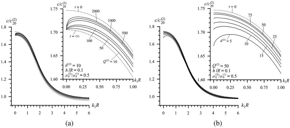
Figure 19: Dispersion curves obtained for various values of the parameter  $Q^{(2)}$  under a fixed value of the parameter  $d^{(2)}$  ( $= 10$ ) (a) and for various values of the parameter  $d^{(2)}$  under a fixed value of the parameter  $Q^{(2)}$  ( $= 50$ ) (b) in the E.V. case under  $\mu_0^{(2)}/\mu_0^{(1)} = 0.5$  and  $h/R = 0.1$ .
