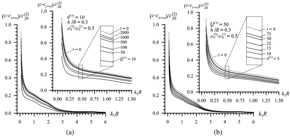
Figure 29: The influence of the parameter  $Q^{(1)}$  under a fixed value of the parameter  $d^{(1)}$  ( $= 10$ ) (a) and of the parameter  $d^{(1)}$  under a fixed value of the parameter  $Q^{(1)}$  ( $= 50$ ) (b) on the wave propagation velocity in the second mode in the V.E. case under the dispersive attenuation case and under  $\mu_0^{(2)}/\mu_0^{(1)} = 0.5$  and  $h/R = 0.3$ .
