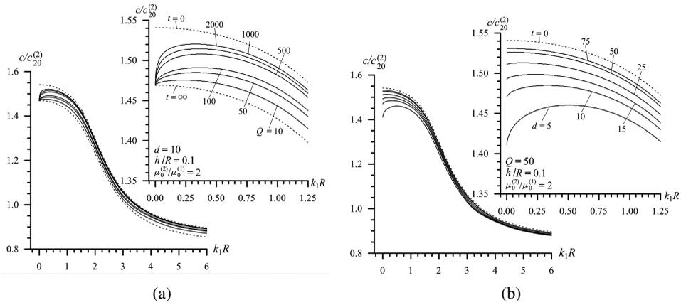
Figure 10: Dispersion curves obtained in the case considered in Fig. 7 under  $\mu_0^{(2)}/\mu_0^{(1)} = 2$  and  $h/R = 0.1$ .
