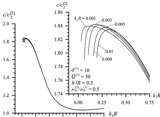
Figure 28: The influence of the “attenuation order”  $k_2R$  on the cut off values of  $k_1R$ , i.e. on the values of  $(k_1R)_{c.f.}$  in the case considered in Fig. 27.
