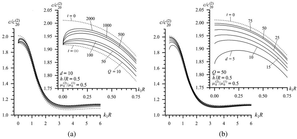
Figure 9: Dispersion curves obtained in the case considered in Fig. 7 under  $h^{(1)}/R = 0.5$ .
