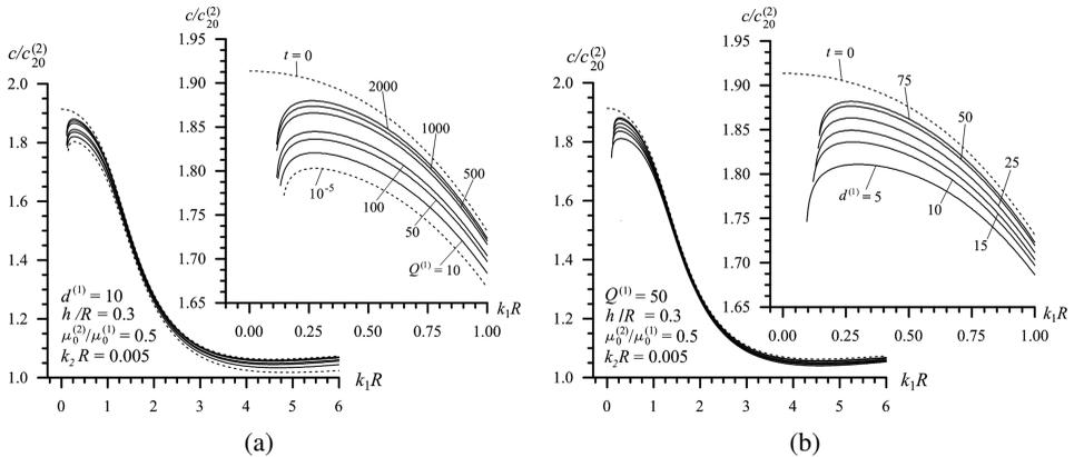
Figure 27: Dispersion curves obtained in the non-dispersive attenuation case under  $k_2 R = 0.005$  in the V.E. case for various values of the parameter  $Q^{(1)}$  under a fixed value of the parameter  $d^{(1)}$  ( $= 10$ ) (a) and for various values of the parameter  $d$  under a fixed value of the parameter  $Q (= 50)$  (b) in the V.E. case under  $\mu_0^{(2)}/\mu_0^{(1)} = 0.5$  and  $h/R = 0.3$ .
