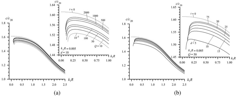
Figure 5: Dispersion curves constructed in the non-dispersive attenuation case for the homogeneous solid cylinder under various values of the parameter  $Q$  for a fixed value of the parameter  $d$  ( $= 10$ ) (a) and for various values of the parameter  $d$  for a fixed value of the parameter  $Q$  ( $= 50$ ) (b) in the case where  $k_2 R = 0.005$ .
