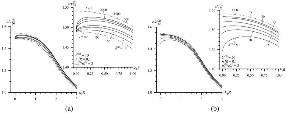
Figure 23: Dispersion curves obtained in the case considered in Fig. 19 under  $\mu_0^{(2)}/\mu_0^{(1)} = 2$  and  $h/R = 0.1$ .
