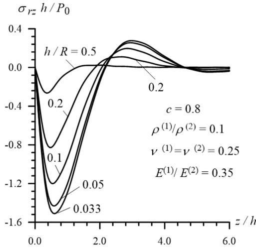
**Figure 18:** The distribution of the shear stress  $\sigma_{rz}$  with respect to the coordinate  $z/h$  in Case 1
