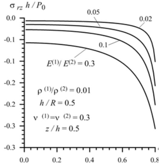
**Figure 15:** The influence of the modulus of elasticity of the cylinder material on the dependence between  $\sigma_{rz}$  and  $c$  in Case 1
