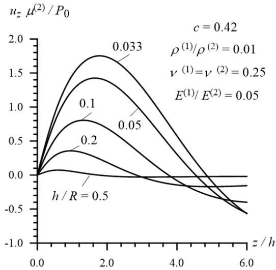
**Figure 23:** The distribution of the radial displacement  $u_z$  with respect to the coordinate  $z/h$  in Case 2
