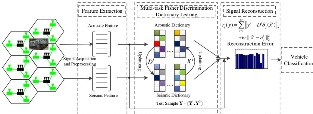
**Figure 1:** The framework of multi-task joint sparse representation based on FDDL for vehicle classification
