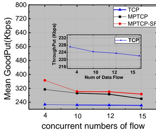
**Figure 8:** Throughput evaluation during long-flows transmission
