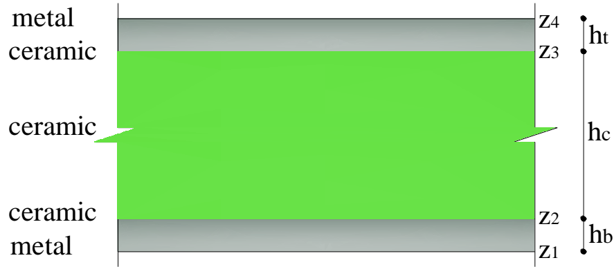
Figure 2: The sandwich plate with FGM sheets and homogeneous core
